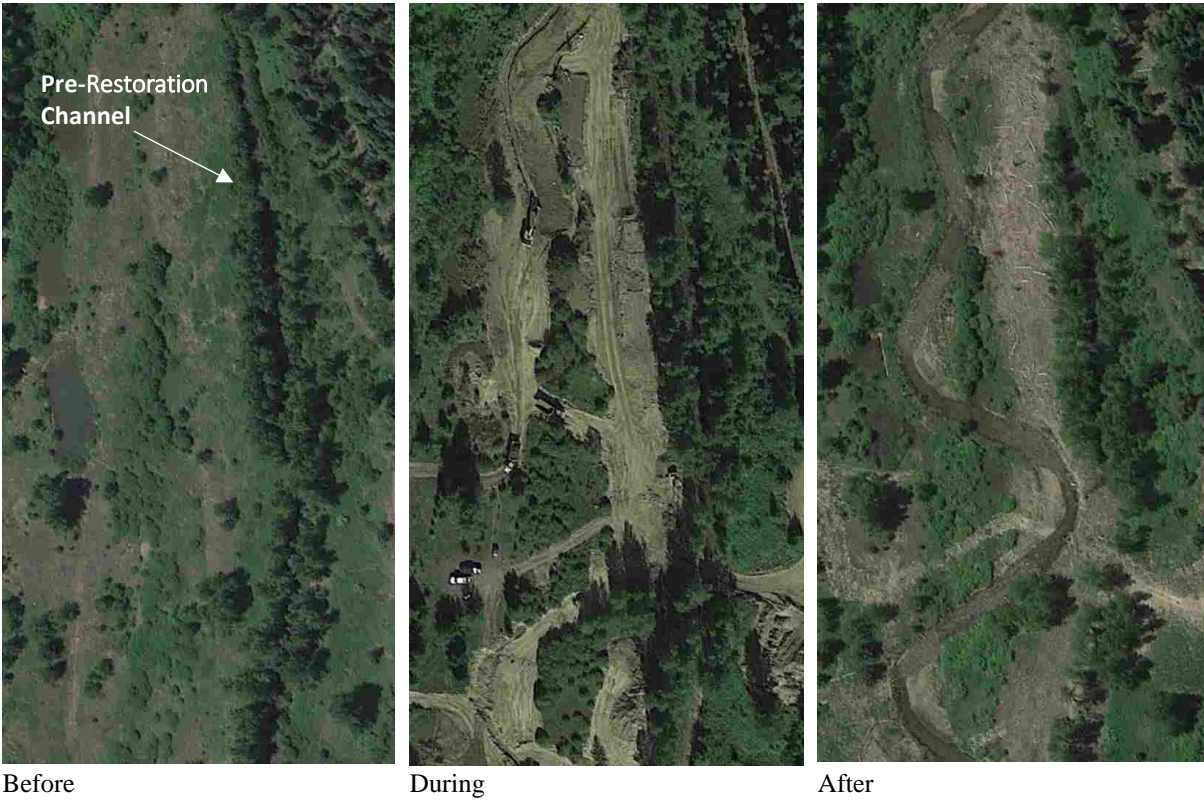
Appendix A. Aerial photographs of a channel reconfiguration in process (Ninemile Creek, MT)
