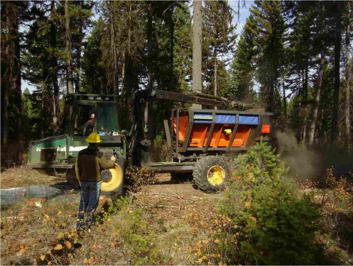
Figure 1.32. Spreader used to distribute biochar in experimental trial in the Lolo National Forest.
