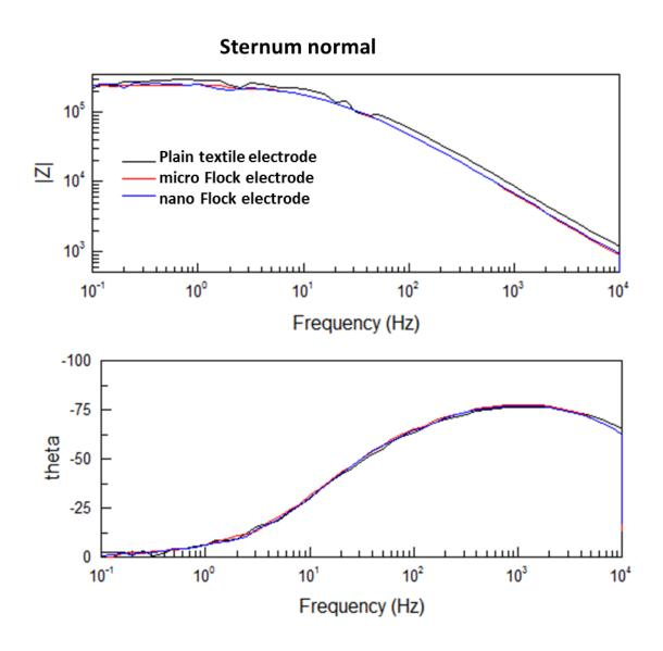
Figure 57: Impedance data from various types of textile based Concentric Ring Electrodes placed on sternum in 3-electrode configuration when subjects were in normal (non-sweaty) condition.
