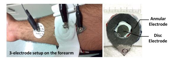
Figure 23: (a) 3-electrode setup on the fore arm with concentric ring electrode (CRE) pair and Ag-AgCl counter electrode, (b) CRE made with flock electrode
