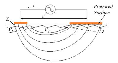
Figure 14: 2-electrode configuration for recording skin-electrode impedance (Z) such that Z = V/i because  $V_1 >> V_2$ ,  $V_3$ .
