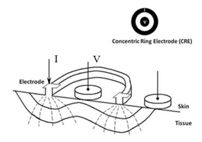
Figure 16: Concentric Ring Electrode: working (current) electrode as annular conductive ring and a voltage taping (non-current carrying) electrode as conductive disc in the center
