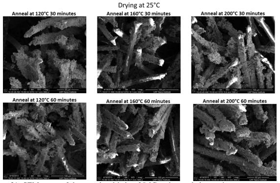
Figure 31: SEM scans of the samples dried at 25 °C and annealed at various temperatures and durations
