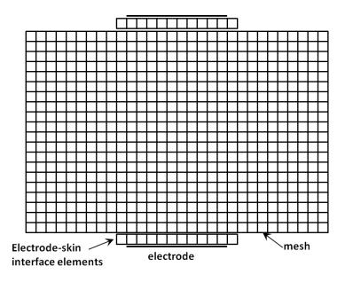
Figure 17: The testing mesh and the electrode-skin interface for a two electrode system
