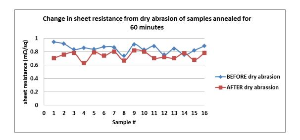
Figure 40: Sheet resistance before and after abrasion under dry conditions of samples fabricated through various temperatures for drying and 60 minutes annealing cycle. The numbering corresponds to the table shown in Figure 36.
