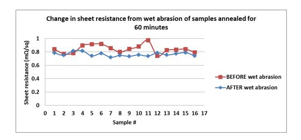
Figure 38: Sheet resistance before and after abrasion under wet conditions of samples fabricated through various temperatures for drying and 60 minutes annealing cycle. The numbering corresponds to the table shown in Figure 36.
