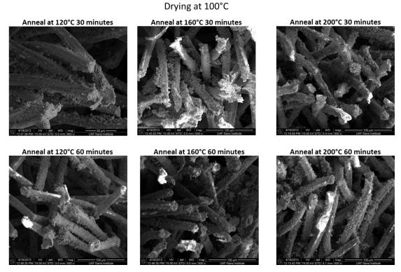
Figure 34: SEM scans of the samples dried at 100 °C and annealed at various temperatures and durations
