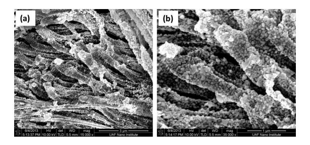
Figure 47: Nanofibers coated with silver nanoparticles
