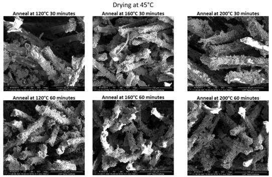
Figure 32: SEM scans of the samples dried at 45 °C and annealed at various temperatures and durations
