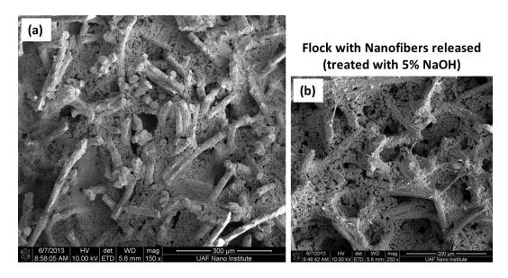
Figure 46: Evolution of the hierarchical structure: The micro pillars (a) treated with 5% NaOH to etch off the polylactic acid matrix polymer to expose embedded nanofibers rendering the micro pillars nanotextured (b)
