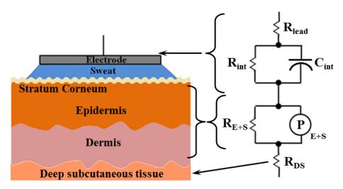
Figure 13: Model of electrode-skin interface for dry electrode and equivalent electrical circuit.
