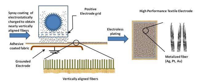
Figure 10: Electrode fabrication technique: Flock application by electrostatic method and then Electroless plating
