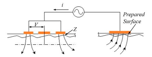
Figure 15: 3-electrode configuration with a non-current carrying electrode to isolate the voltage drop across the skin from that of the whole system.
