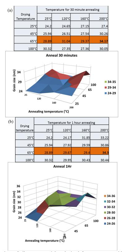
Figure 30: Grain sizes of silver nanoparticles obtained from processes with different drying temperature and annealing temperature for (a) 30 minutes annealing (b) 1hr annealing
