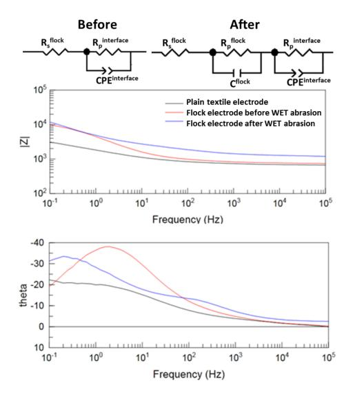
Figure 41: Contact impedance measurement before and after wet abrasion along with the equivalent (model) circuit for both cases.
