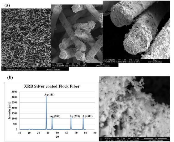
Figure 29: (a) SEM scans of silver flocked electrode with fiber dia. ~10μm. (b) XRD of silver coated flocked nylon fibers corresponding to face center cubic (fcc) silver
