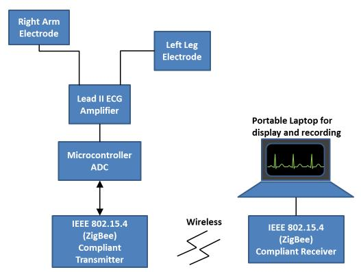
Figure 27: Block diagram of the transmission module for a portable ECG measurement system: ECG signal is amplifier by a differential analog amplifier, the analog to digital converter (ADC) and ZigBee module transmits the signal to a receiver connected to a laptop computer.
