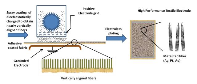
Figure 19: Electrode fabrication technique: Flock application by electrostatic method and then Electroless plating
