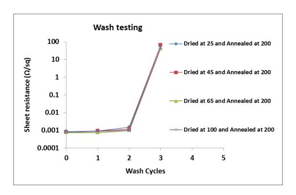
Figure 43: Impedance data from wash testing: (a) sheet resistance (b) contact resistance
