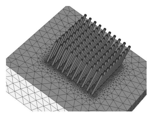
Figure 25: Physics controlled mesh generated for the model geometry. The mesh density was increased at the interface of the microfibers and the agar gel for higher resolution and accuracy in mapping of the electrical currents
