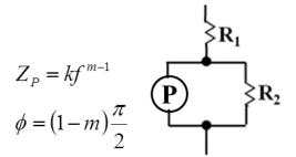
Figure 12: Polarization impedance element as a part of R-[RC] circuit
