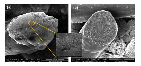
Figure 44: Polylactic acid nanocomposite fiber made of 1500 polypropylene nanofibers (dia. <200nm) in a matrix (sea) of polylactic acid: (a) nanocomposite fiber cross-section with nanofibers visible in the inset (b) polylactic acid dissolved to release the embedded nanofibers
