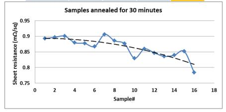
Figure 35: Variations in sheet resistance of flock electrode samples fabricated using different drying temperatures and different temperatures for 30 minute annealing process
