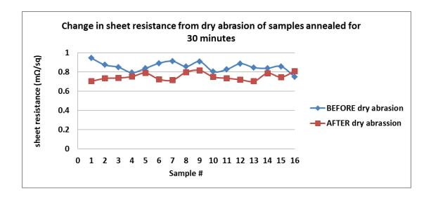
Figure 39: Sheet resistance before and after abrasion under dry conditions of samples fabricated through various temperatures for drying and 30 minutes annealing cycle. The numbering corresponds to the table shown in Figure 35.
