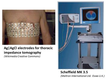
Figure 7: Commercial EIT system: Electrode setup and Scheffield MK 3.5
