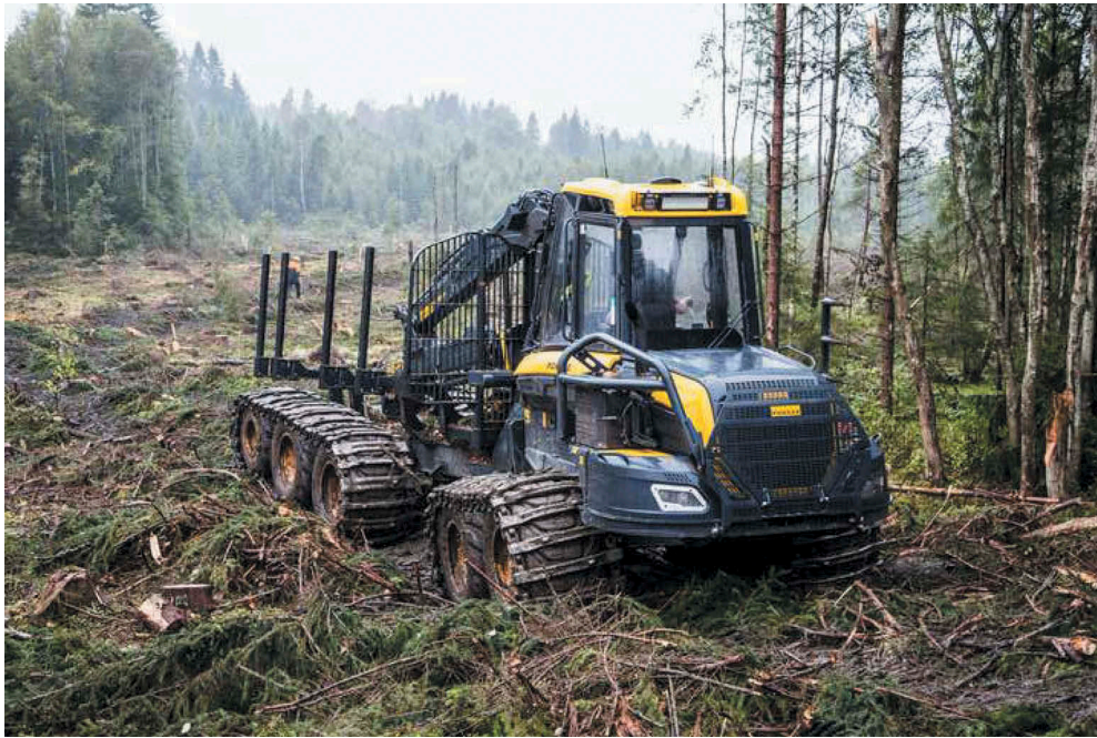
Figure 1. The Ponsse Buffalo 10-wheeled forwarder used in the field test (photo R. Dalen) showing a standard track on the front bogie and a combi-track on the rear bogie. The auxiliary axle is seen behind the rear bogie and has variable axle pressure when in use.
