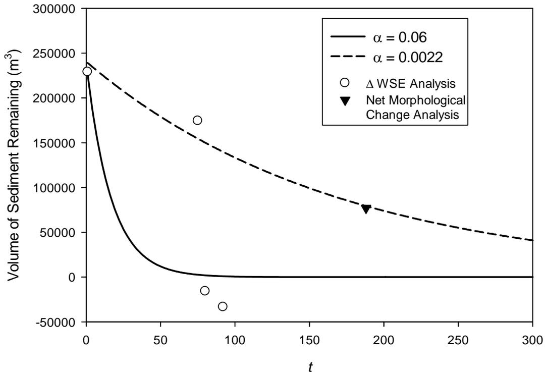
Figure 27. Exponential decay functions fit through the  $\Delta$ WSE and net morphological change estimates of volumetric erosion. The pattern of erosion in the time period examined does not appear to exponential. However, subsequent years may prove that erosion may show an exponential decay pattern.
