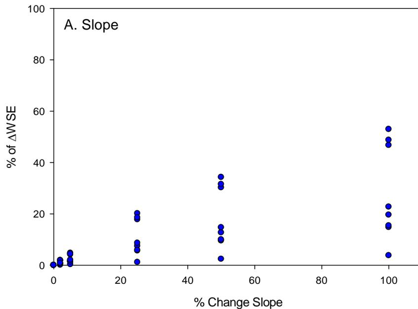
Figure 28. Sensitivity analysis of  $h$  to changes in A. Slope, and B. Manning's  $n$ . A 100% increase in Manning's  $n$  could account for ~10% of  $\Delta$ WSE, while a 25% change in slope may account for 20% of  $\Delta$ WSE.
