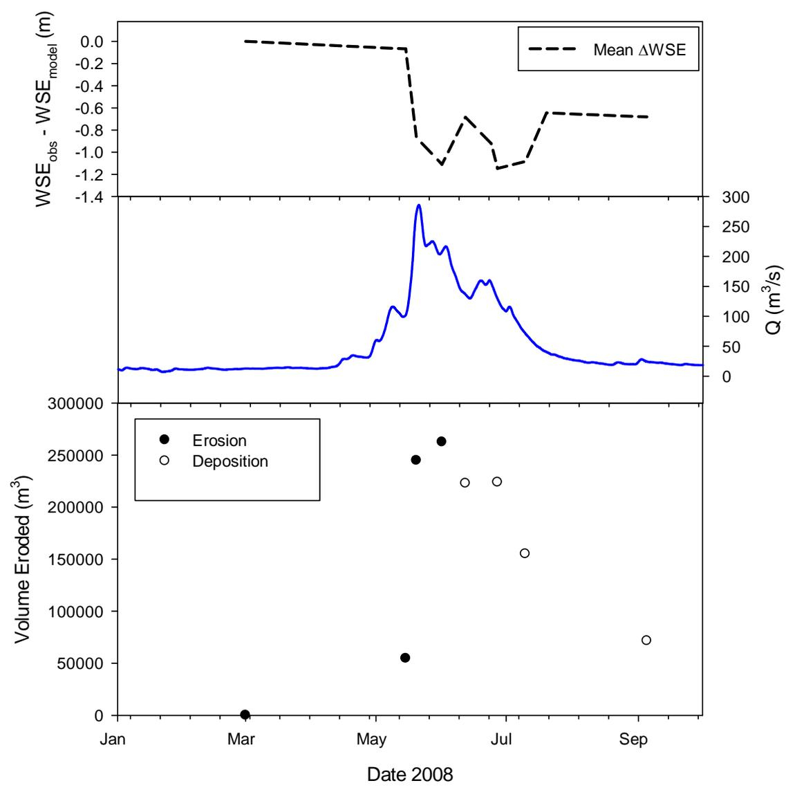
Figure 25. Mean  $\Delta WSE$ , 2008 hydrograph and volumetric erosion through the hydrograph. Solid points show increasing erosion, and white points show sediment deposition during the falling limb of the hydrograph.
