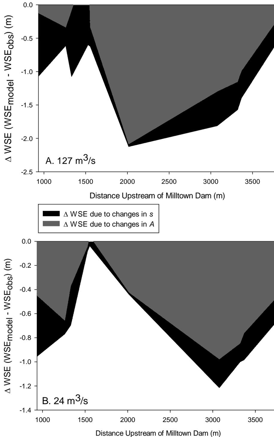
Figure 29.  $\Delta WSE$  with sensitivity analysis results incorporated for (A) 6/27/08 ( $Q = 127 \text{ m}^3/\text{s}$ ) and (B) 9/5/08 ( $Q = 24 \text{ m}^3/\text{s}$ ). The potential maximum dilutive effects of a 100% change in slope is illustrated by these two  $\Delta WSE$  analyses. The black area represents the proportion of  $\Delta WSE$  that can be explained by a 100% change in slope. The black and grey areas added together represent the total  $\Delta WSE$ .
