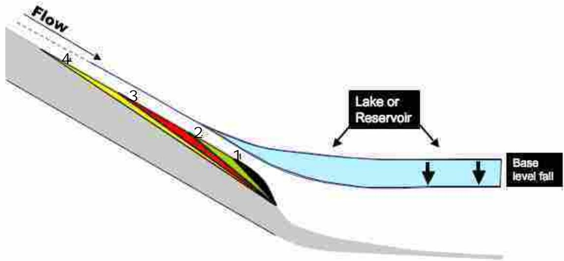
Figure 1. Idealized diagram of base level fall from a reduction in lake or reservoir elevation. Progression of upstream erosion through time ( $t = 1$  through 4). Adapted from Galay 1983.
