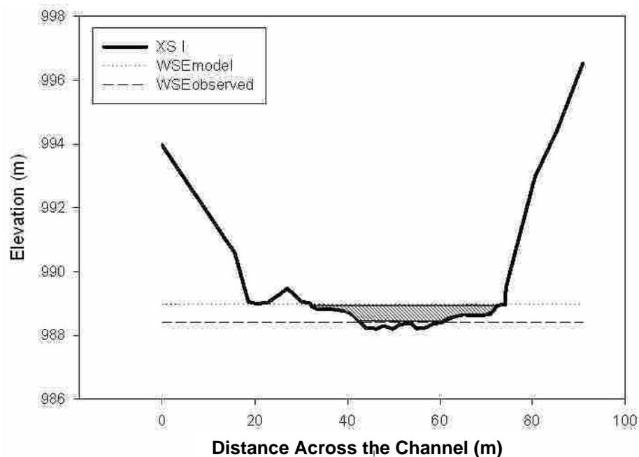
Figure 11. Pre-erosion cross sectional topography for Cross Section I. Dotted line is  $WSE_{model}$ , dashed line is  $WSE_{obs}$ . Erosion of the shaded cross sectional area between the two lines is the hypothesized mechanism causing a deviation between the observed and modeled water surface elevations.
