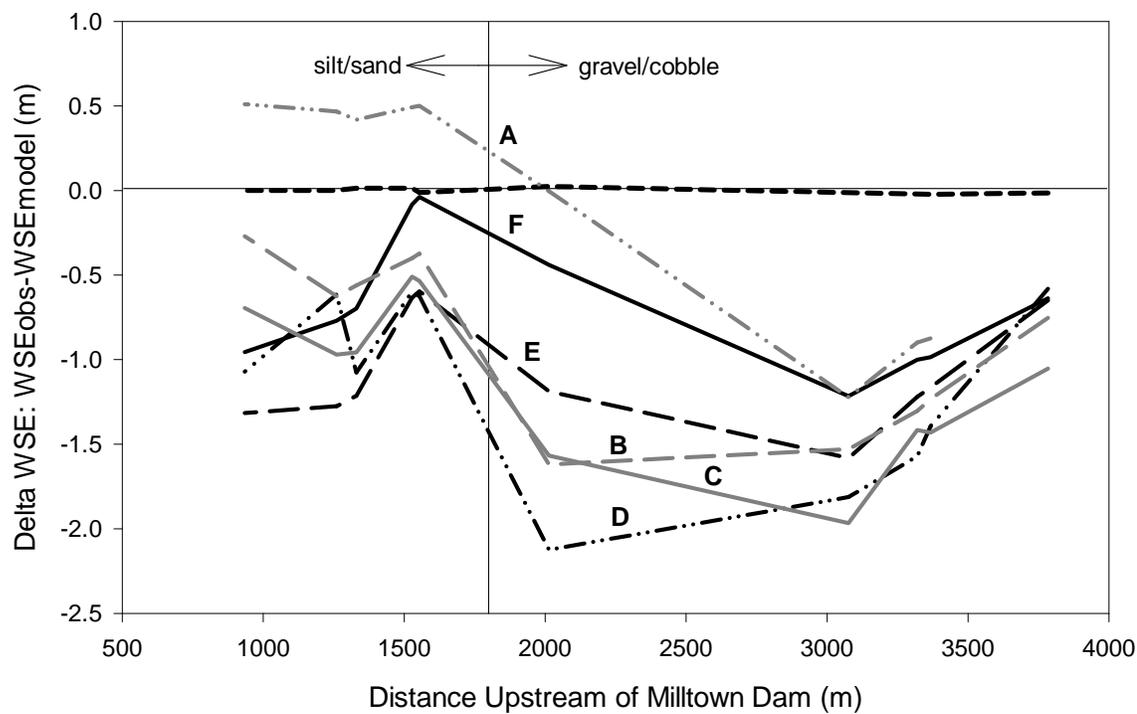
Figure 24.  $\Delta WSE$  curves throughout the hydrograph plotted against distance upstream. The bold dashed calibration line shows  $WSE_{model}$  fits the  $WSE_{obs}$  at Spring 2008 baseflow. A, the gray dash-dotted line, is the earliest date and associated discharge modeled. F, the solid black line, is the latest discharge modeled, from 9/5/08. Note the vertical line representing the gravel-sand transition in the Spring of 2008.
