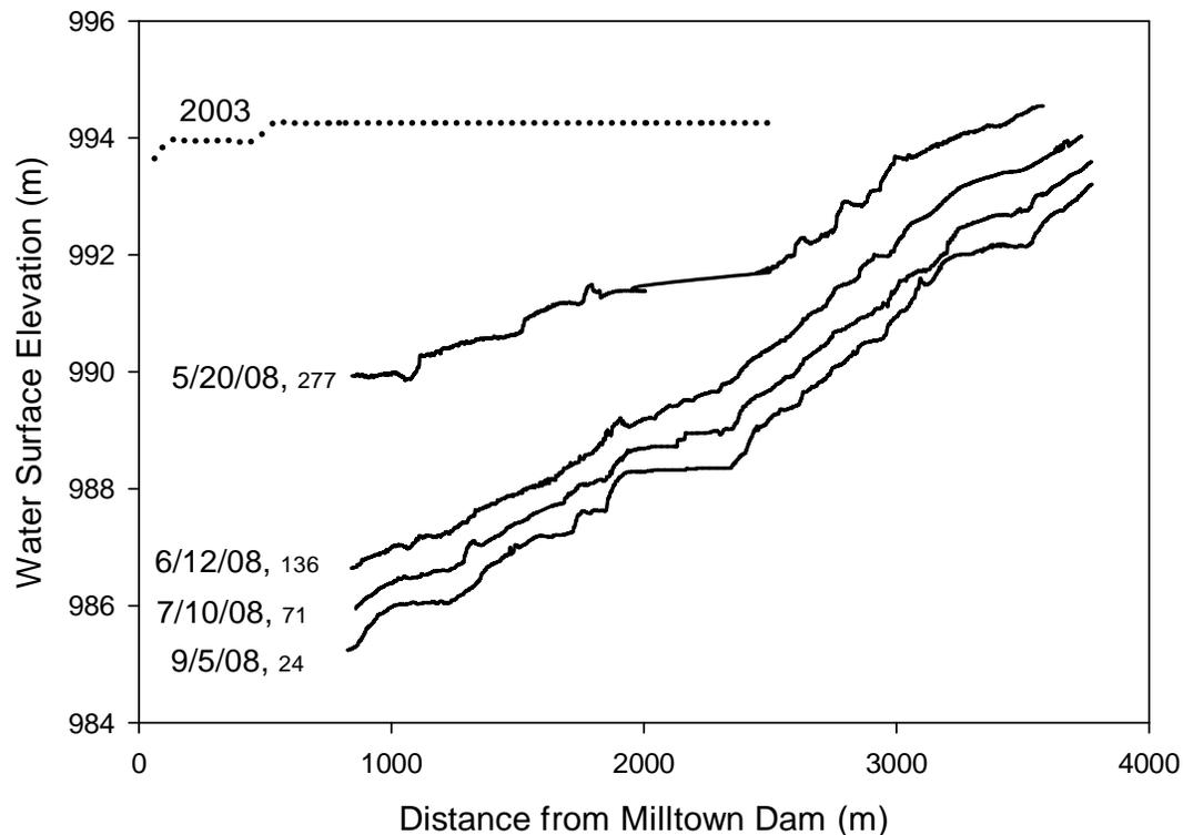
Figure 26. Water surface profiles throughout the 2008 hydrograph shown with the 2003 reservoir water surface. Dates for water surface profiles surveyed in 2008 listed with discharge ( $\text{m}^3/\text{s}$ ).
