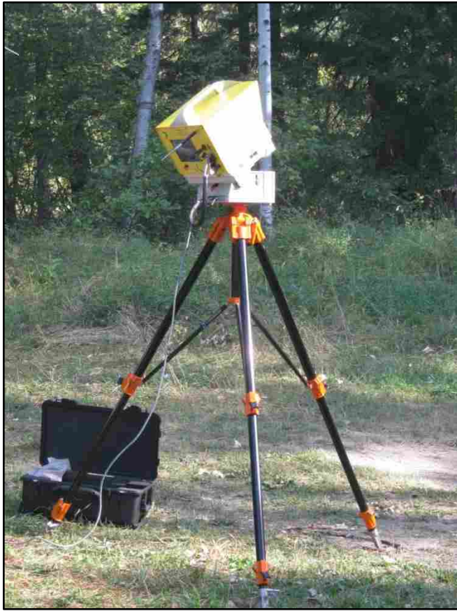
Figure 6. The Optech ILRIS 3 6 D HD terrestrial laser scanner. The laser and scan head (yellow) are mounted on a pan-tilt unit that permits bi-directional rotation, and sit atop a level tripod. The laser is powered by a battery pack and scanning is controlled remotely through a hand-held device. Data is written to a USB that connects at the rear panel of the scan head.
