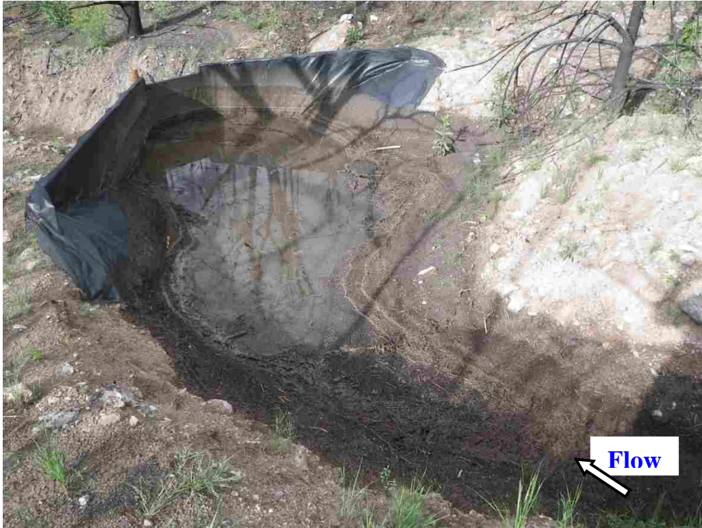
Figure 18. In treated catchment G, this sediment retention structure captured 2.55 Mg of sediment that was transported past three empty or partially full straw bale check dams that sat lowest in the channel closest to the catchment outlet, during the 8 Jul 2011 storm.
