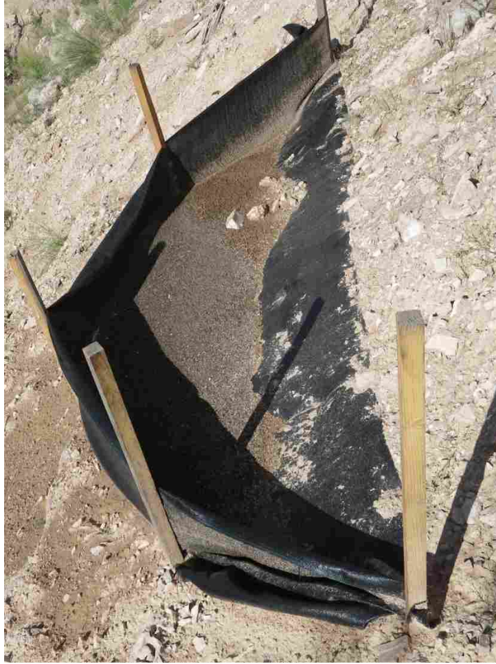
Figure 14. Hillslope fence G captured total sediment yield from an 11 mm (0.4 in) 27 \text{ mm hr}^{-1} ( 1.1 \text{ in hr}^{-1} ) rain event on 8 Jul 2011 that was less than a 1-year I_{10} recurrence interval event.
