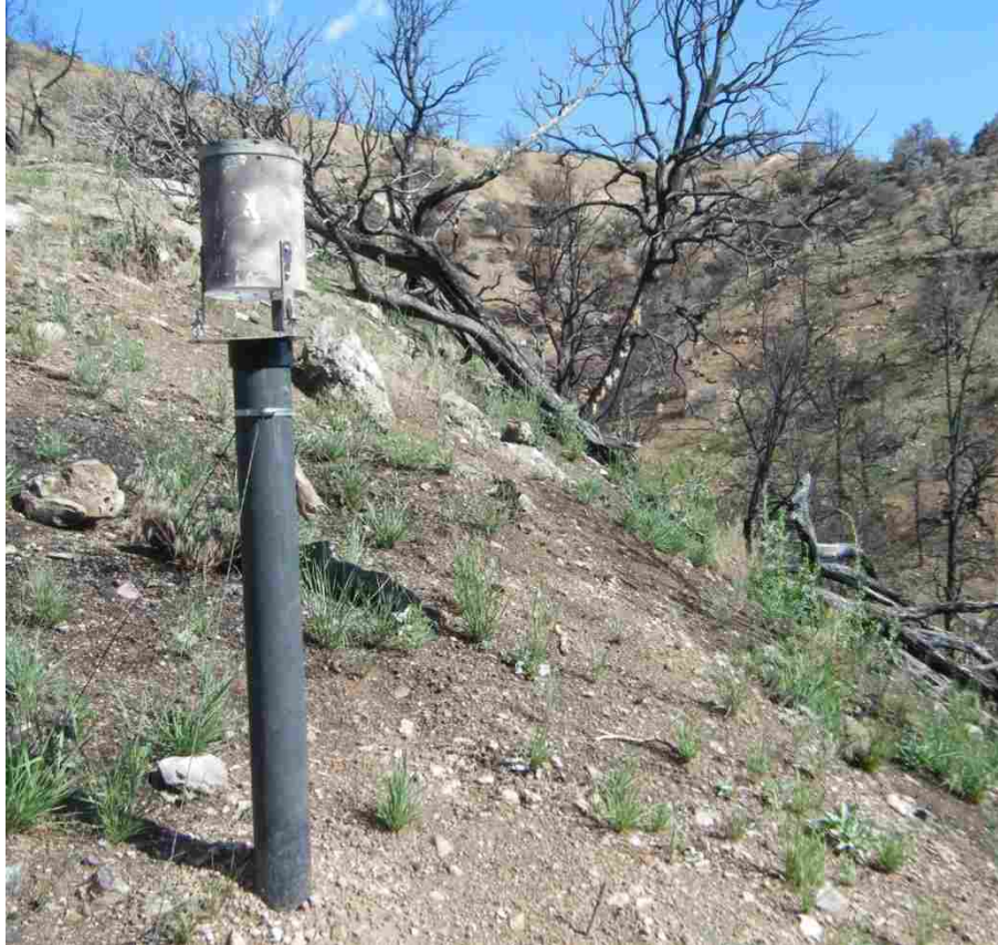
Figure 9. Tipping bucket rain gauge (~20 cm [8 in] opening) set level to the ground and located roughly half way up catchment ridge (monitored catchment in background). The rain gauge was mounted to a plate of sheet metal attached to the top of a 10 cm (4 in) diameter PVC post. The hollow PVC post was buried 45 cm (~18 in) into the ground, filled to the brim with soil, and secured with three guy-wires spaced at 120° that were attached to the post 140 cm (~55 in) from the ground surface and anchored at the ground with rebar to reduce systematic error of wind disturbance tipping the recording bucket.
