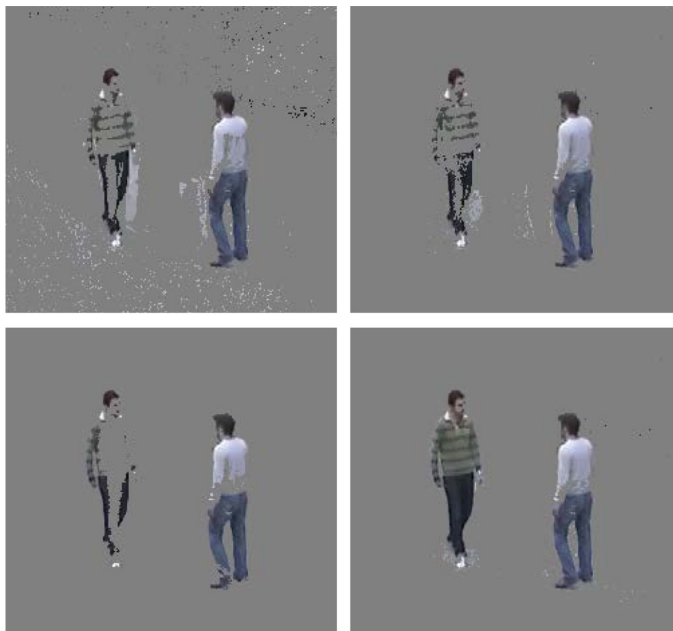
Figure 12. Residuals of the video data, for classical PCA (upper left), Spearman correlation (upper right), Huber's \psi (lower left), and wrapping (lower right).
