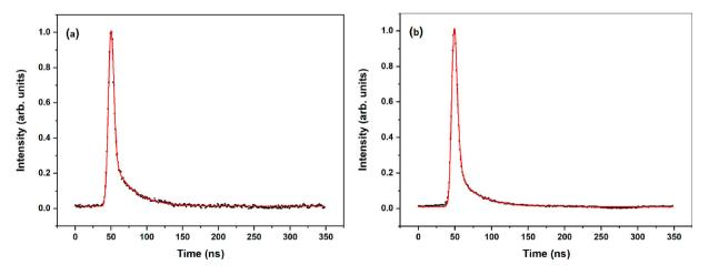
**Figure 3.** (1 + 1') R2PI decay curves of the (a) *syn/cis* (A) and (b) *anti/cis* (B) conformations of methyl sinapate after excitation at their vibrationless origin transition (31059.8 and 31170.1 cm<sup>-1</sup>, respectively). The red traces are fits of the decays to the convolution of a Gaussian profile with a biexponential decay with decay times (relative contribution) for *syn/cis* (a) of 1.8 ns (0.93) and 27.0 ns (0.07), and for *anti/cis* (b) 3.1 ns (0.93) and 29.2 ns (0.07).
