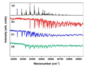
**Figure 4.** (a) (1 + 1') R2PI excitation spectrum of the methyl sinapate-H<sub>2</sub>O cluster monitoring the mass of the methyl sinapate ion. The asterisks in the spectrum indicate the probe frequencies used in (b-d) to obtain conformation-specific absorption spectra with UV-UV depletion spectroscopy at 30238.0 (b), 30374.8 (c) and 30324.6 (d) cm<sup>-1</sup>.
