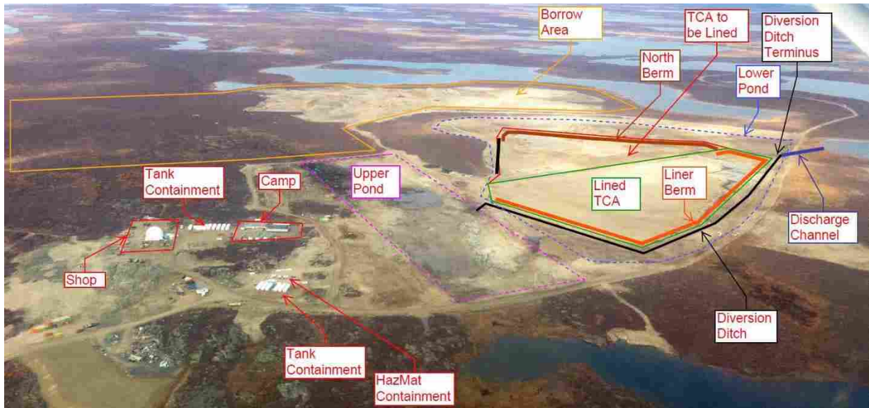
Figure 2- 3: Aerial photo of un-vegetated sites during reclamation phase at Tundra Gold Mine, NWT, Canada. Photo is showing Upper Pond (pink outline) and Lower Pond (blue outline), which were previous tailings area. Lower Pond still contains tailings, but they are now capped and covered with rock material. Borrow Area, is an open quarry that rock material was excavated from to use on the tailings. Photograph obtained from Report Phase 2 Remedial Action Plan, Tundra Mine Site (Golder 2008).
