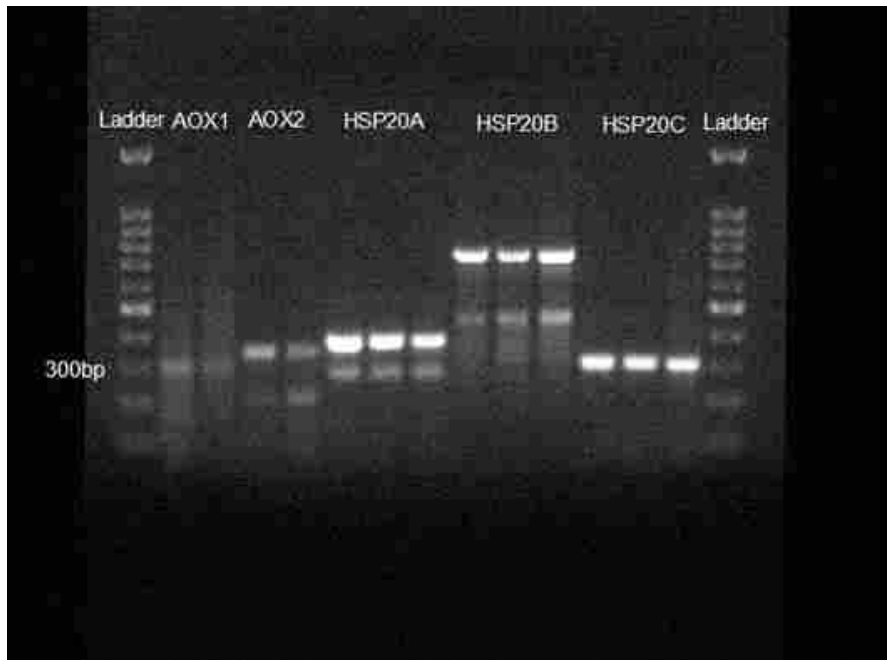
Figure 6: Agarose gel electrophoresis (2% agarose) of PCR amplified products using AOX and HSP20 primers and T. californicus isolated DNA. 3 \mu L of DNA ladder (GeneDirex, 100bp DNA Ladder Ready To Use), and the subsequent wells were loaded with 12 \mu L of each PCR sample. The gel was run at 80 V for approximately 1 hour and 20 minutes. Expected product sizes are displayed in Table 1.
