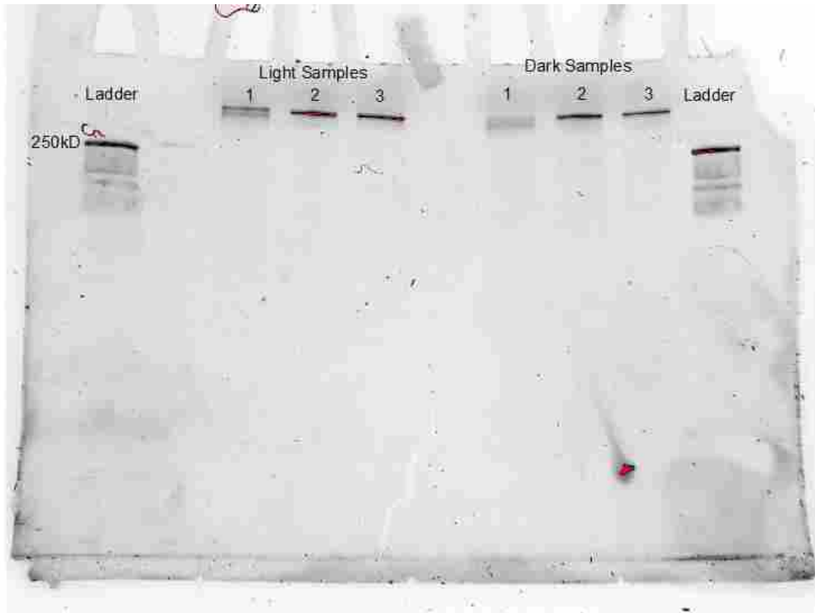
Figure 31: Chronic light and dark exposure protein samples run on reducing SDS-PAGE post transfer onto a TransBlot Turbo Mini-size Nitrocellulose (Bio-rad) membrane using the TransBlot Turbo Blotting System (Bio-rad).
