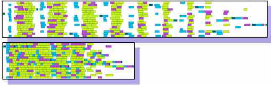
Figure 1. Comparison of fork-join and task parallelism. Execution trace of the same algorithm implemented using fork-join parallelism (top) and task-based parallelism (bottom). The bottom version executes in less time because worker threads can continue executing tasks as soon as the tasks’ dependencies have been satisfied. From [244].
