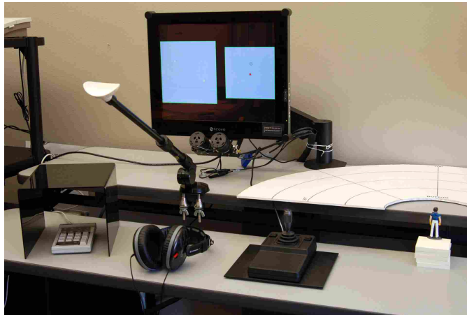
FIGURE 6. The experimental setup including the visual display, headphones, chin-rest, keypad, joystick, and a physical representation of the audio transformation scheme. Image from Hornof et al. (2008).
