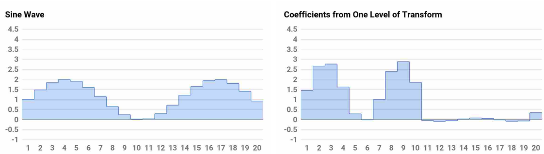
Figure 1. Demonstration of information compaction of wavelets. The input is a discrete sine wave with 20 data points (left), and the output is 20 wavelet coefficients (right). The magnitude of the wavelet coefficients is proportional to their information content.
