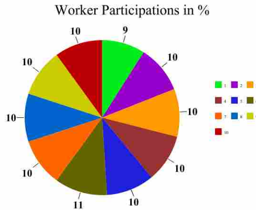
FIGURE 5.5. Apache Spark workers participation in SSSPInc for update batch \alpha = 0.1\% , \beta = 0.1\% for Friendster graph.
