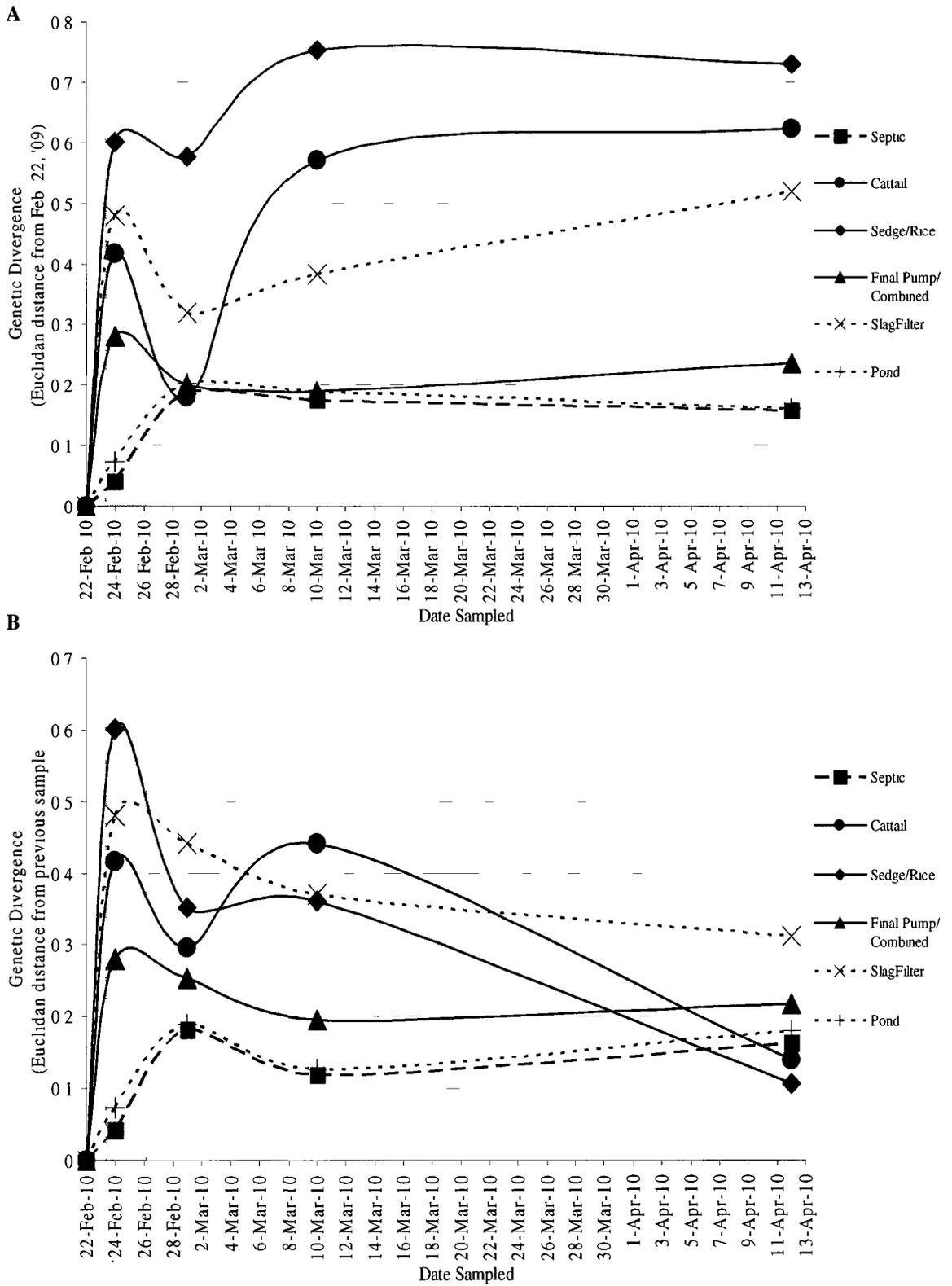
**Figure 5.12.** Genetic divergence based on Euclidian distances of untransformed DGGE profiles from the field-scale CW. A) Divergence from the Feb. 22<sup>nd</sup> sample, for each sample at each location and B) Divergence from the previous sample.
