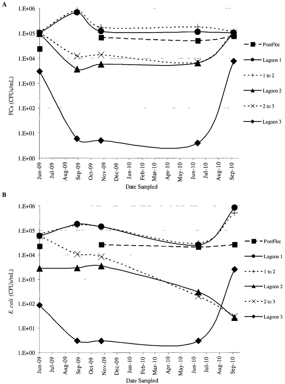
**Figure 6.1.** Graphical representation of FCs and *E. coli* enumerated in the industrial-scale treatment lagoon. A) Faecal coliform and B) *E. coli* enumeration on mFC + 1% Rosolic acid and mFC + 1% BCIG, respectively. Counts were completed between 24 and 48 hours of incubation in a water bath @ 44.5°C.
