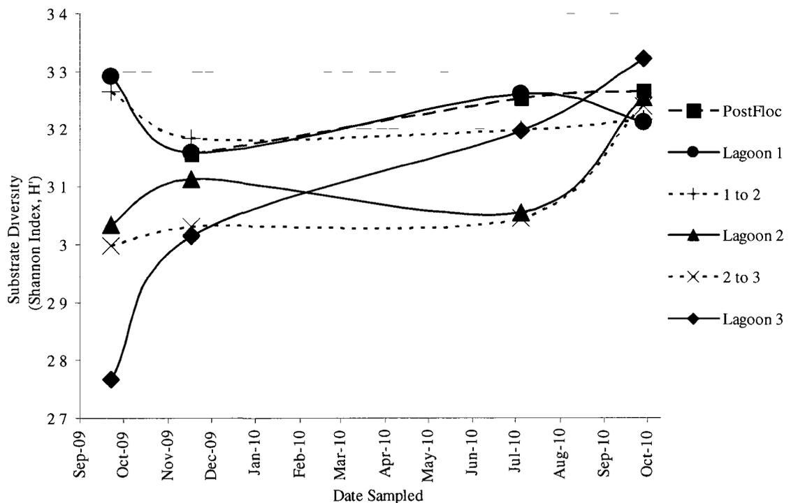
**Figure 6.4.** Substrate diversity (Shannon  $H'$ ) calculated from the industrial-scale treatment lagoon CLPP after 72 hours of incubation at 22°C
