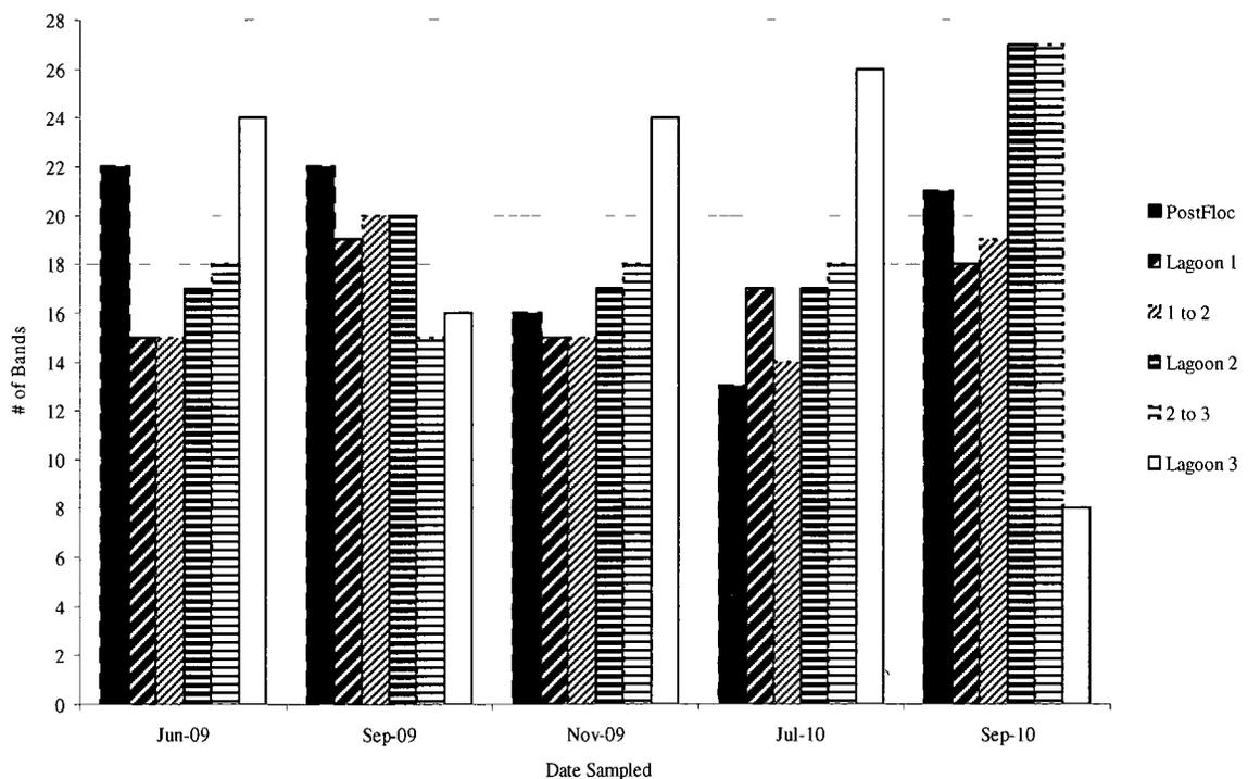
**Figure 6.9.** DGGE-based community richness (# of bands) from the industrial-scale treatment lagoon. PCR-DGGE was done using the DNA extracted from the 10 mL centrifuged pellet.
