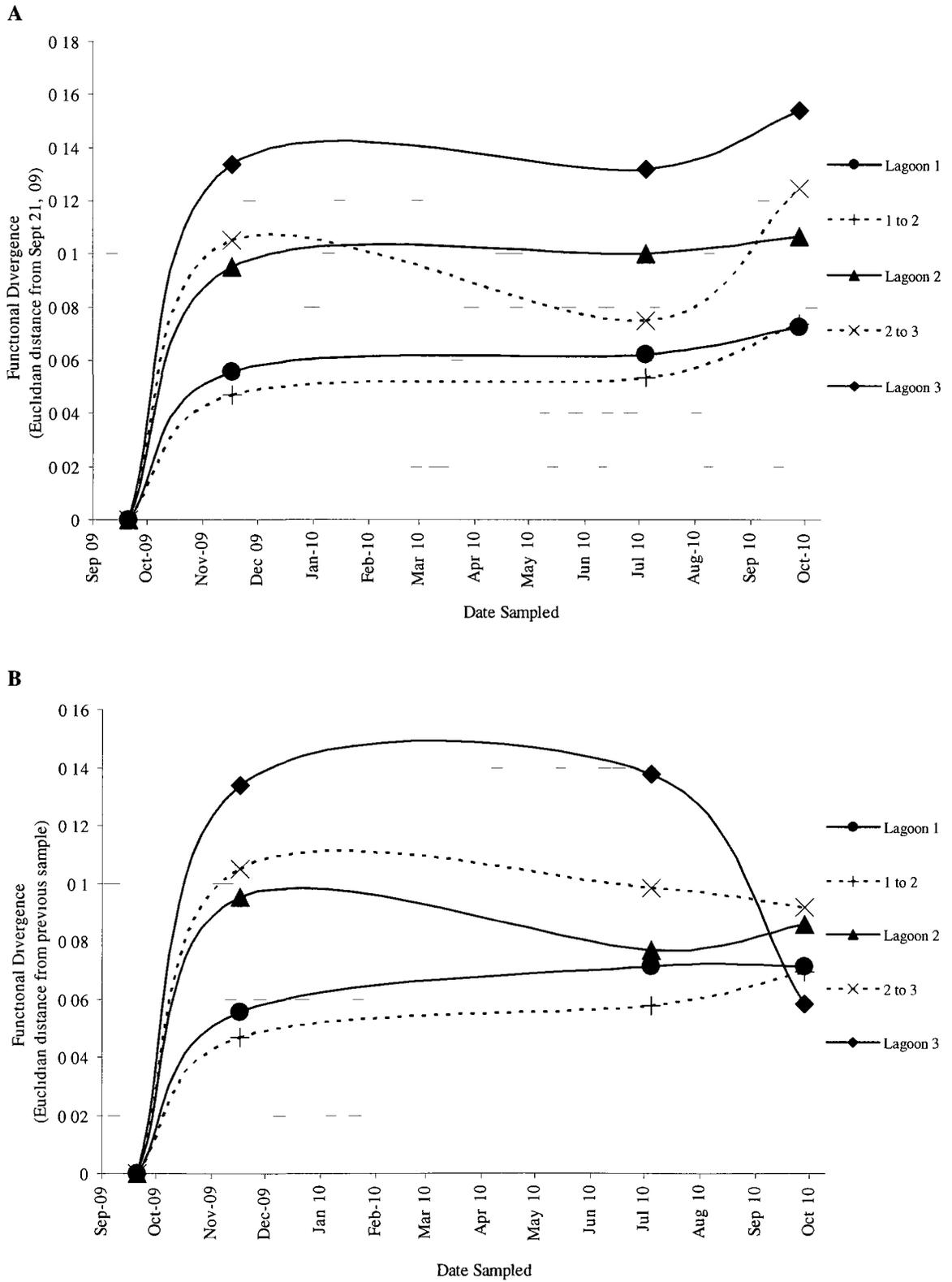
**Figure 6.5.** Functional divergence based on Euclidian distances of untransformed CLPP profiles from the industrial-scale treatment lagoon A) Divergence from the sample taken on Sept 21<sup>st</sup> and B) Divergence from the previous sample The PostFloc location was not included in this calculation
