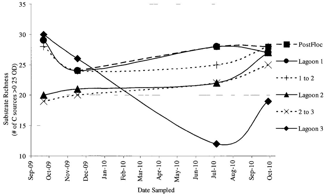
**Figure 6.3.** Substrate richness calculated from the industrial-scale treatment lagoon CLPP after 72 hours of incubation at 22°C
