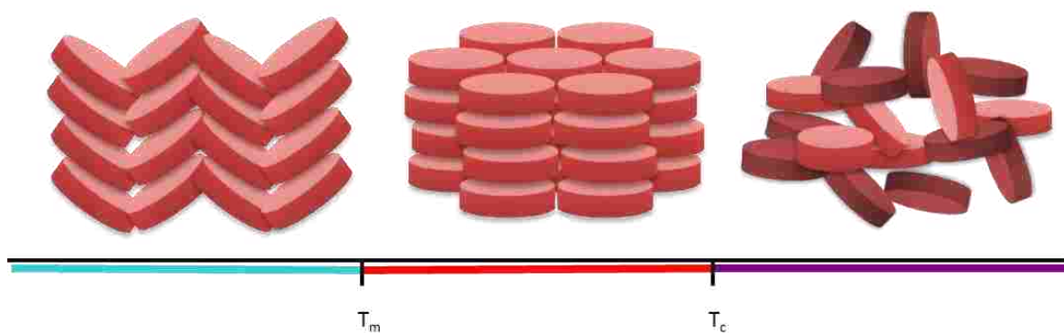
Figure 1-3: Typical transitions for discotic liquid crystals. From left to right we see the crystal state, the liquid crystal state (in this case a columnar phase) and the isotropic liquid state.
