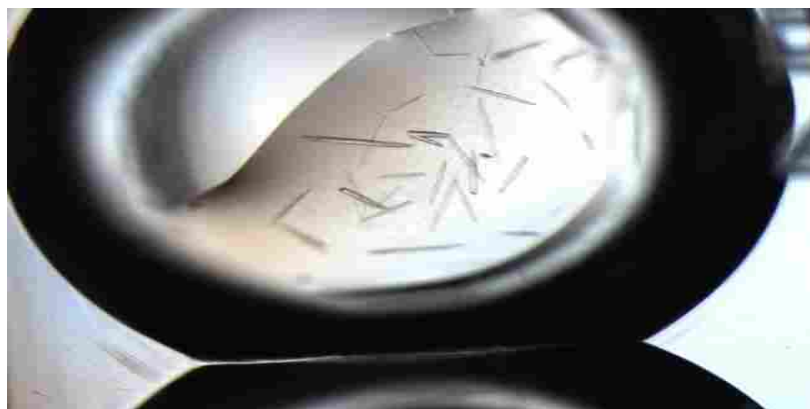
Figure 27: Crystal growth of BFO 2294 in MCSG 2 over seven days. The condition was B4: 1.8 M \text{NaH}_2\text{PO}_4/\text{K}_2\text{HPO}_4 pH 8.2
