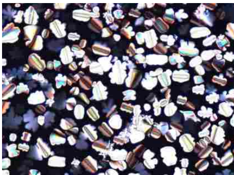
Figure 4-9: Polarized optical micrograph of 30 % TNF / 70 % DBA mixture at 59 °C on cooling at a rate of 10 °C·min -1 and taken at 200x magnification.
