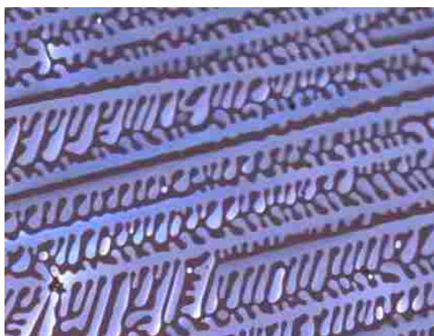
Figure 4-6: Polarized optical micrograph of 1:1 HAT-6/TNF mixture at 212 °C on cooling at a rate of 10 °C·min -1 and taken at 200x magnification.
