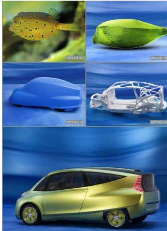
Figure 21: DaimlerChrysler Bionic Car Development Process
