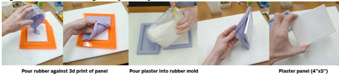
Figure 5: Process of using a 3D printed part to create a rubber mold
