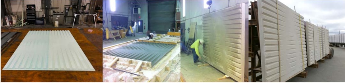
Master panel CNC-cut from high density foam
