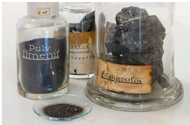
FIGURE 1 Ilmenite, rich in iron and titanium, was the starting material for the production of titanium white pigment, which was co-organised by Peder Farup, professor at NTH. The samples shown in the picture are from the historical collections of the Department of Chemistry at NTNU. © NTNU/ Åge Hojem, NTNU University Museum.
