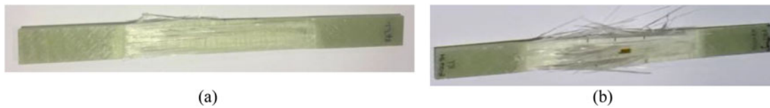
Figure 10. Failure mechanisms for longitudinal tensile tests. The samples show failure breakage and matrix cracking as the white region. Failure of fiber and matrix are generalized on the whole sample. For both composite systems the samples failed abruptly. (a) LEO system. (b) Sicomin system.
