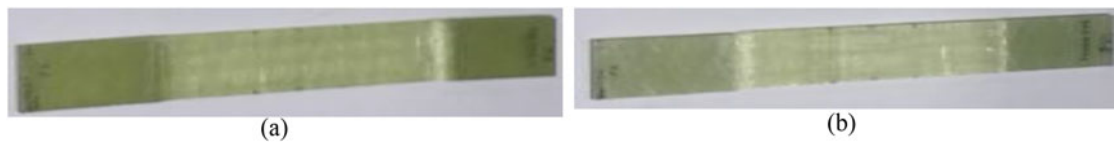
Figure 13. Failure mechanisms for transverse tensile tests. Both systems presented matrix failure as the white region of them. The samples did not split in two parts, given the existence of longitudinal fibers on the second ply of the laminate. (a) LEO system. (b) Sicomin system.
