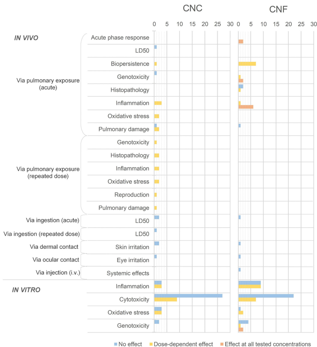
Figure 1. Systematic review of toxicity results of CNC and CNF. The length of the bars refers to the number of investigated materials (i.e. each with specific physicochemical properties) per endpoint, represented in terms of observed effect. As certain studies looked at multiple materials, a similar table relating to the number of studies having been conducted per endpoint can be found in the Supplementary material Figure S1 .
