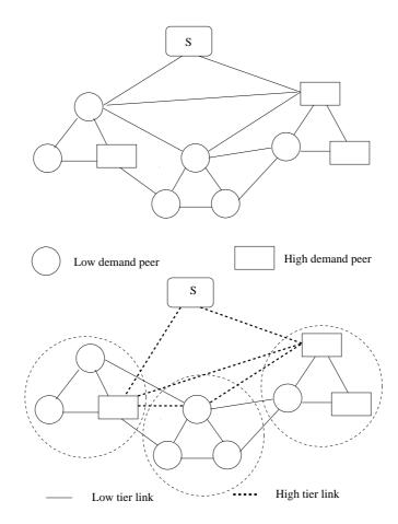
Figure 4.6: Tiered overlay of a P2P streaming system
