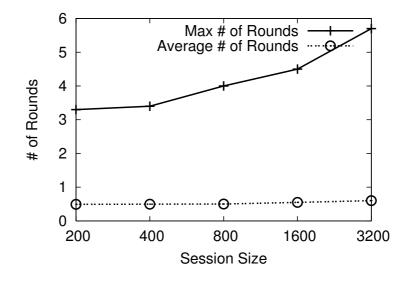
Figure 6.5: Convergence Speed of HFP: HFP converges fast even with the increase of system size.
