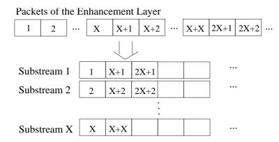
Figure 3.4: A simple way to divide the enhancement layer into X substreams.
