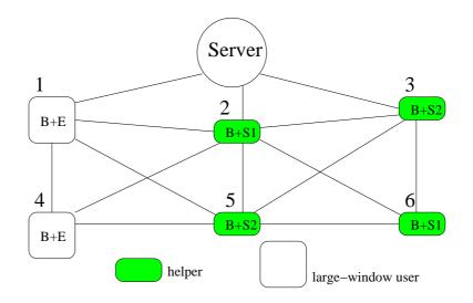
Figure 3.3: With PFS, *every* small-window user is a helper, and helps to forward a *substream* of the enhancement layer. In this figure, the whole enhancement layer (denoted by E) is divided into two substreams (denoted by S1 and S2).
