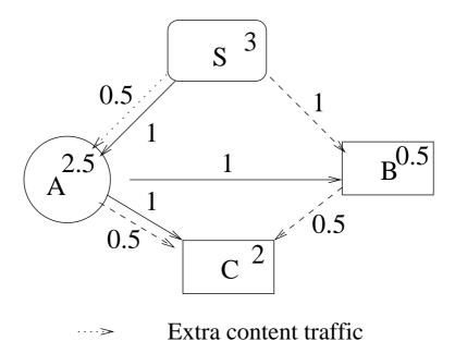
Figure 4.3: Bandwidth allocation cannot always solve the problem, and extra forwarding is required. Peer A downloads the enhancement layer not required by itself, then streams it to peer C, as C cannot get the enhancement layer from B at a sufficient streaming rate.
