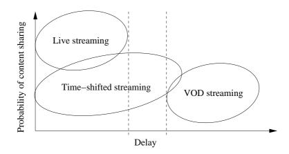
Figure 5.1: Live vs Time-shifted vs VOD streaming.
