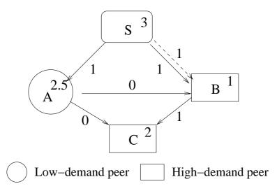
Figure 4.1: An improper upload bandwidth allocation at peers makes the system suffer heavy server load and poor performance. Superscripts of the server and peers indicate their upload bandwidth, and the streaming rate of each link is also marked next to the link.
