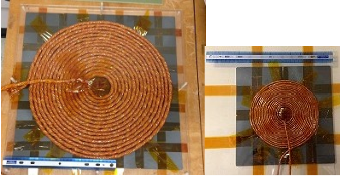
Figure 5.20: Asymmetrical Coupler for 3kW Wireless Charging of EV showing larger Tx(left) and smaller Rx(right).
