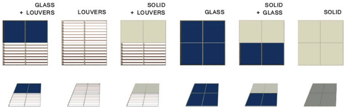
Figure 41: Roof Panel Types
