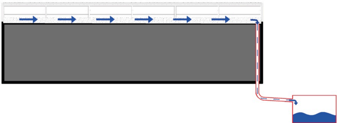
Figure 31: Butterfly Roof System and Flow of Water
