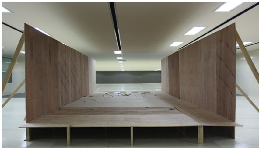
Figure 1. Structure of small-scale simulation model set up at the 30 cm height from the ground.
