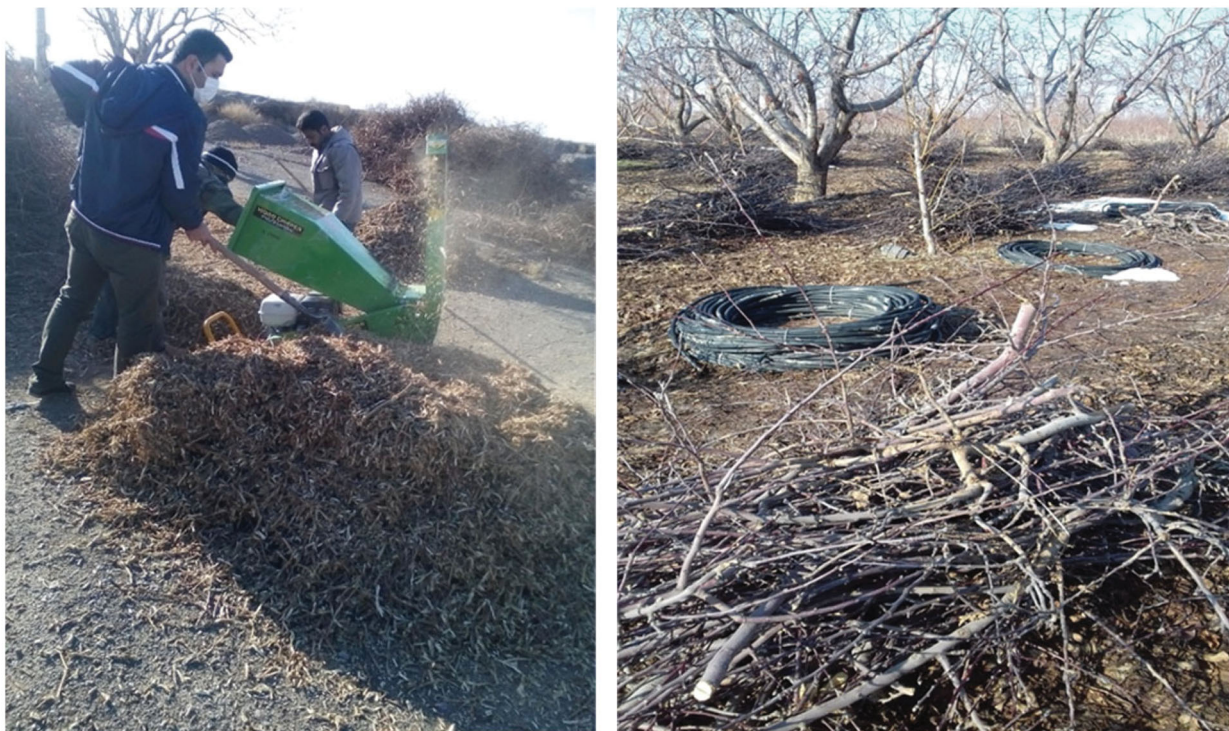
Figure 2. Woody pruning residues of apple trees and processing with chipper KOREN K 17000.
