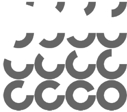
Figure 3. Visual feedback given to the tele-operator in eye-tracking conditions during target selection. The feedback signifies that the current visual fixation point is in the process of being selected. When a completed circle is presented the tele-operator responds with a nod of the head to acknowledge the selection of the intended target.
