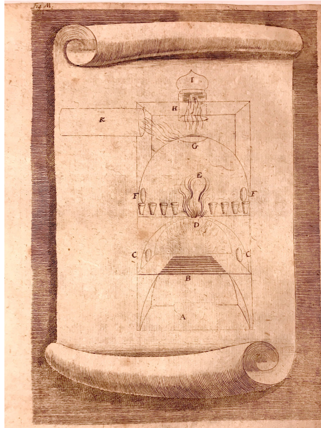
FIGURE 5 A sketch of Kunckel's compendious furnace that contained several small crucibles used for testing (F). Especially noteworthy is the fire channel (K) that could be used to connect to another and smaller furnace. Photo: Thijs Hagendijk.
