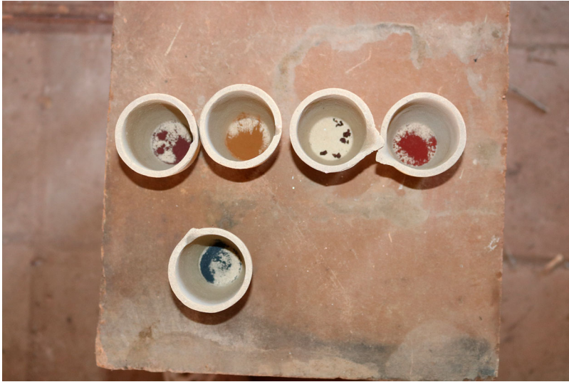
FIGURE 2 An overview of the five different crocus martis . Top row, from left to right: crocus martis prepared with sulphur (chapter 16); crocus martis prepared with vinegar (chapter 17); crocus martis prepared with aqua fortis (chapter 18), and crocus martis prepared with aqua regia (chapter 19). Below: the crocus martis prepared without additives, as described by Kunckel in his commentary. Photo: ARTECHNE/VICARTE.
