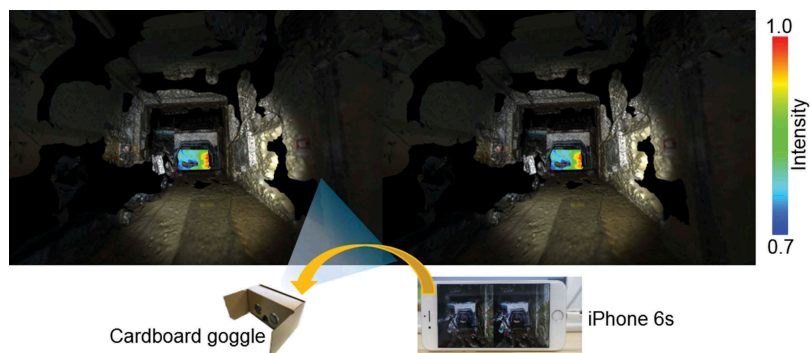
Figure 8. 3-D stereo view of image of radioactive hotspot superimposed on 3-D structural model of inside of reactor building of Unit 1 of the FDNPS.
