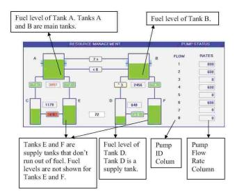
When the resource management task begins, the fuel level for Tanks A and B is at 2500 units. You are to keep the level of fuel from dropping below or above this level as indicated by the marker on either side of these pumps. As time passes, tanks A and B lose fuel. These tanks would eventually become empty without the transfer of additional fuel. Tanks C and D only lose fuel if they are transferring fuel to another tank.
