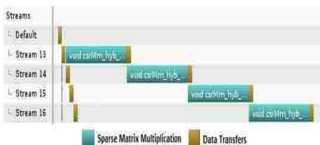
(1) Overlap of computing and data transferring
