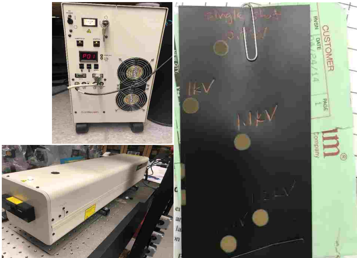
Fig. D. 1 Continuum Nd:YAG laser power supply controller and laser head. The thermal paper shows the beam profile after installation.
