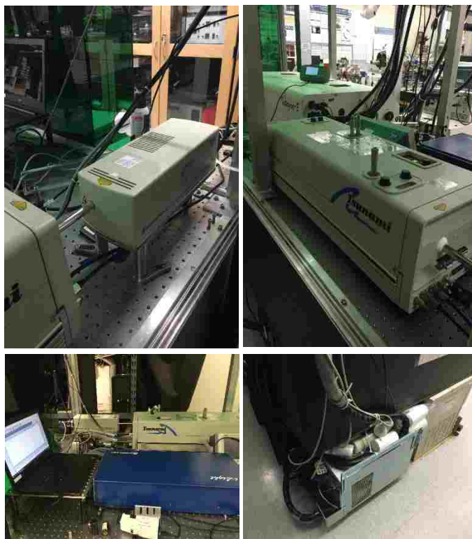
Fig. C. 16 Green laser (Millenia), seed laser (Tsunami), and power supply for green laser. Refer the manual for more details of operation.
