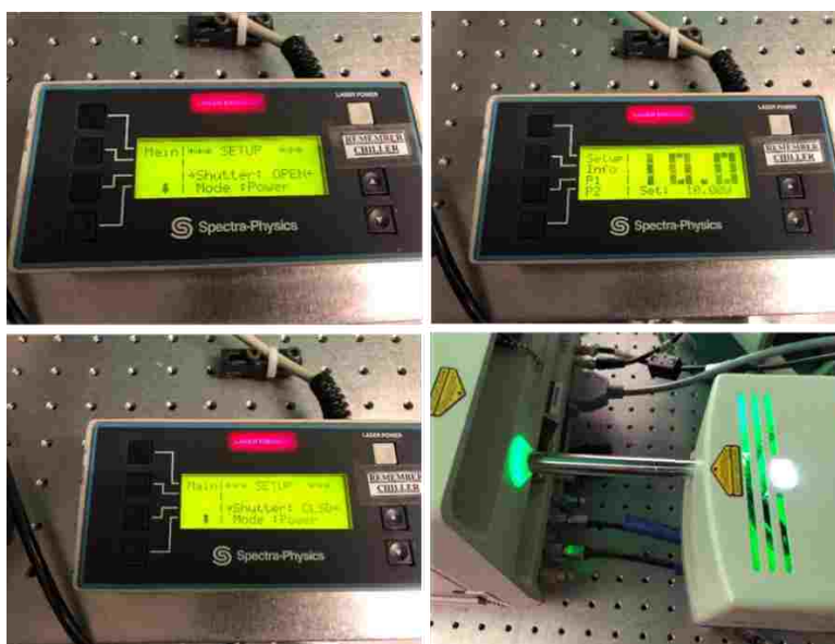
Fig. C. 17 Millenia laser controller and connection between Tsunami and Millenia.
