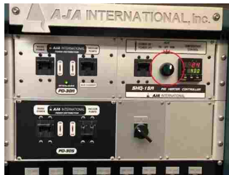
Fig. B. 3 Substrate rotation switch and manual control section.
