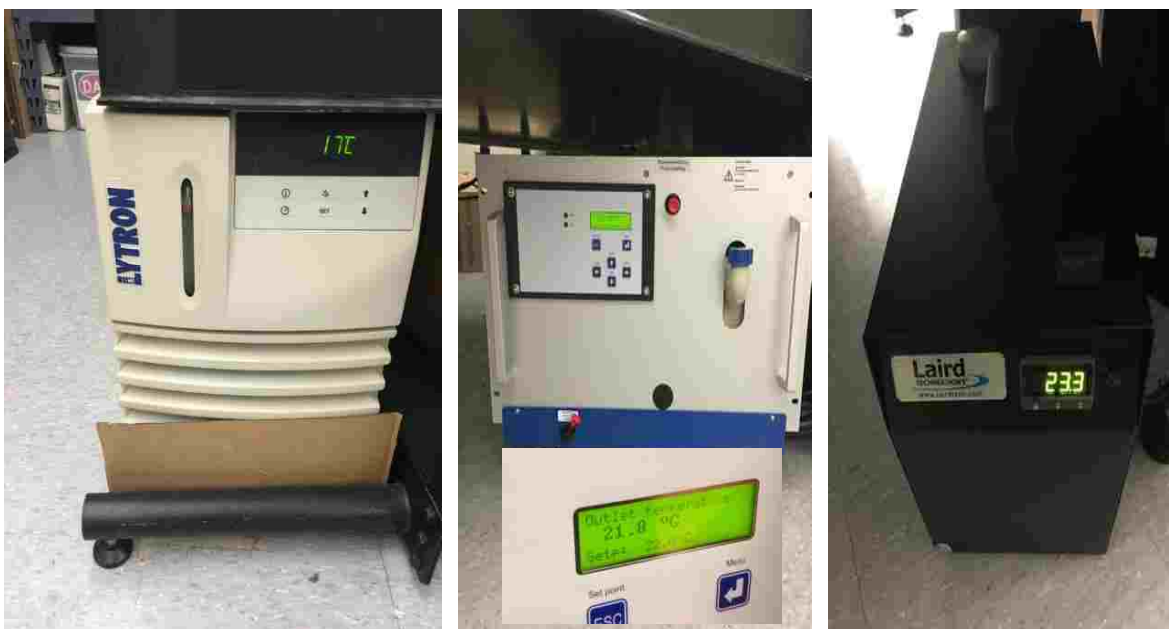
Fig. C. 10 Chillers for Millenia (green) laser, Terra (in Regen, pump), and Tsunami (seed).
