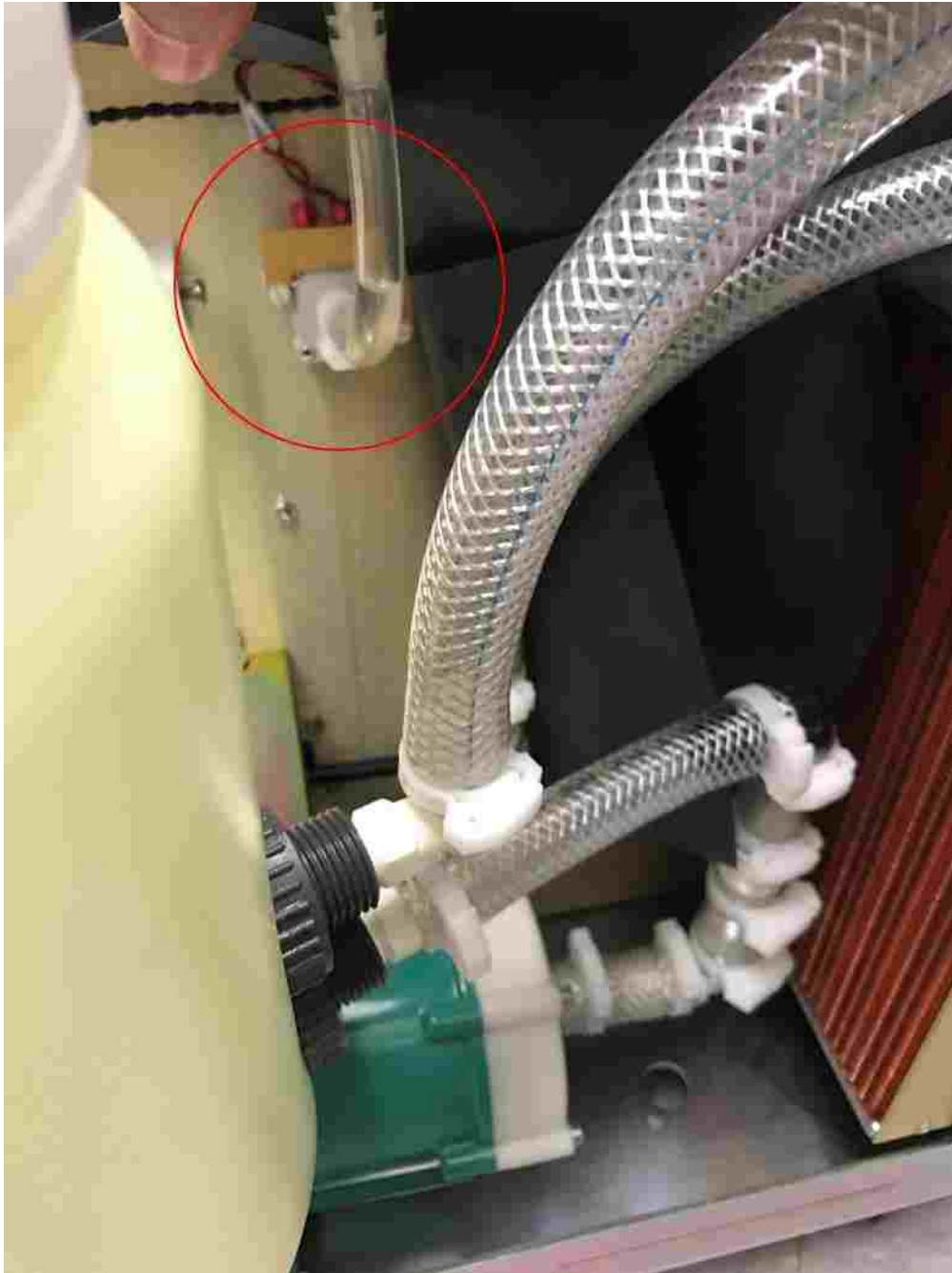
Fig. D. 8 Pressure switch location. Simply unplug the two red wires and hose, and replace the part with the new one.
