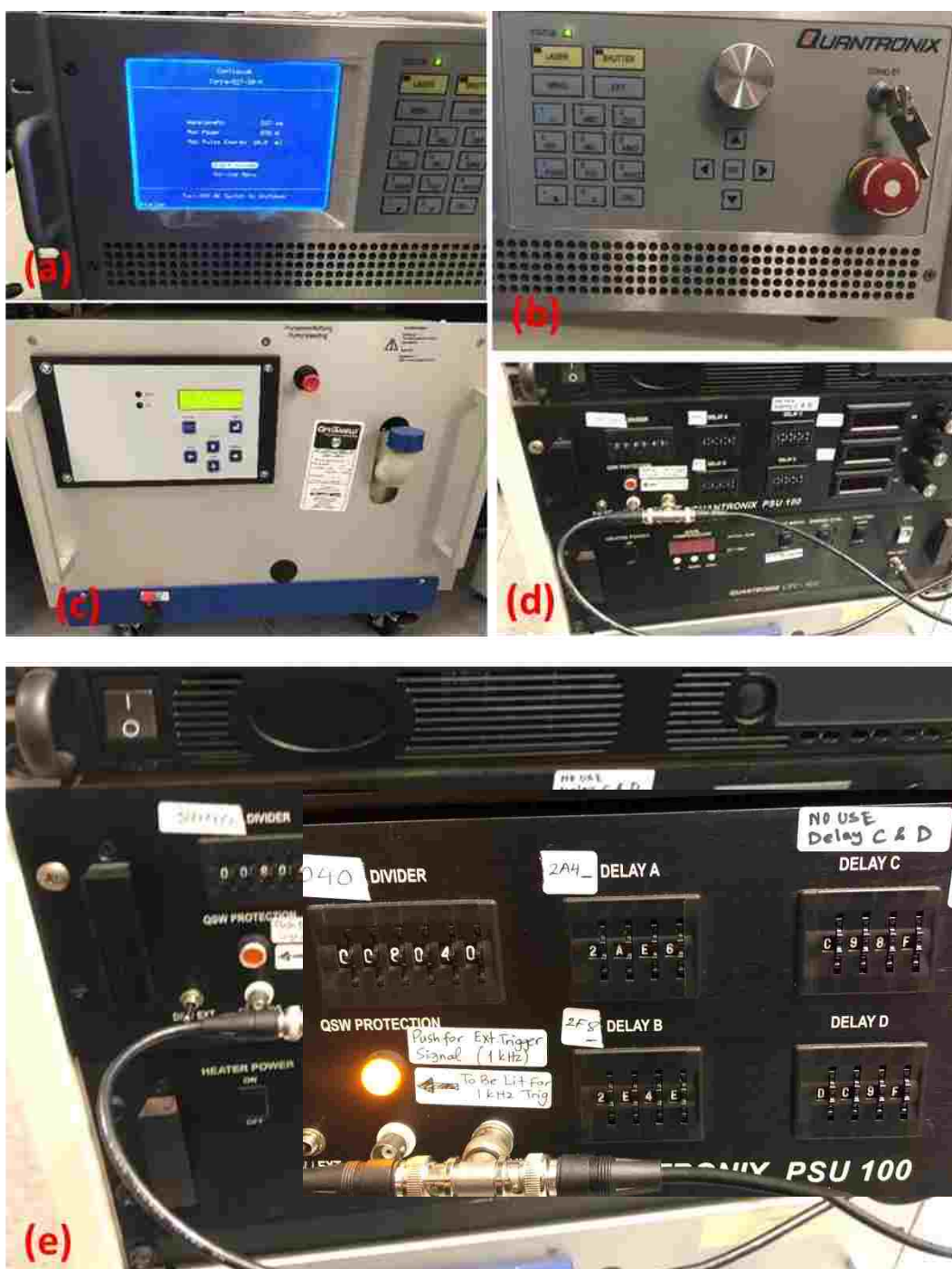
Fig. C. 4 (a), (b) Terra laser controller interface, (c) the chiller, (d) the controller panel for setting up delay, Pockels cell parameters, and frequency selection. (e) Close look of the controller panel.
