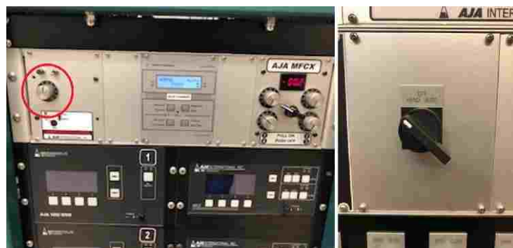
Fig. B. 3 Substrate rotation switch and manual control section.
