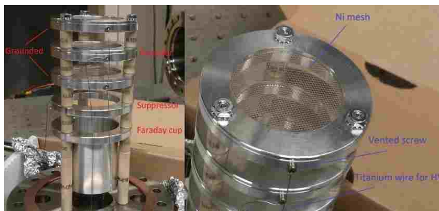
Fig. A. 3 Faraday cup with its components.
