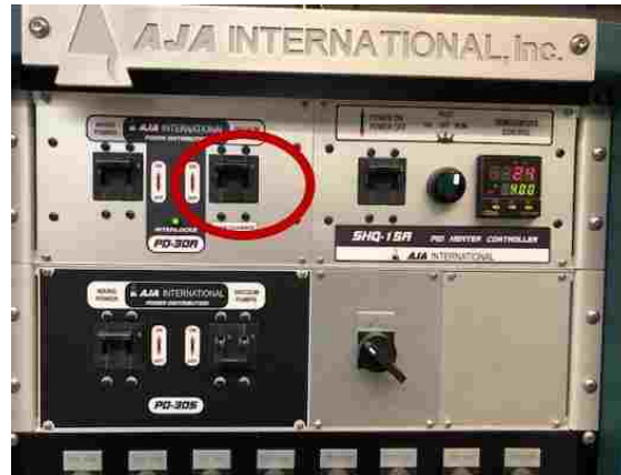
Fig. B. 2 Turbo pump turn ON/OFF switch on the upper panel.
