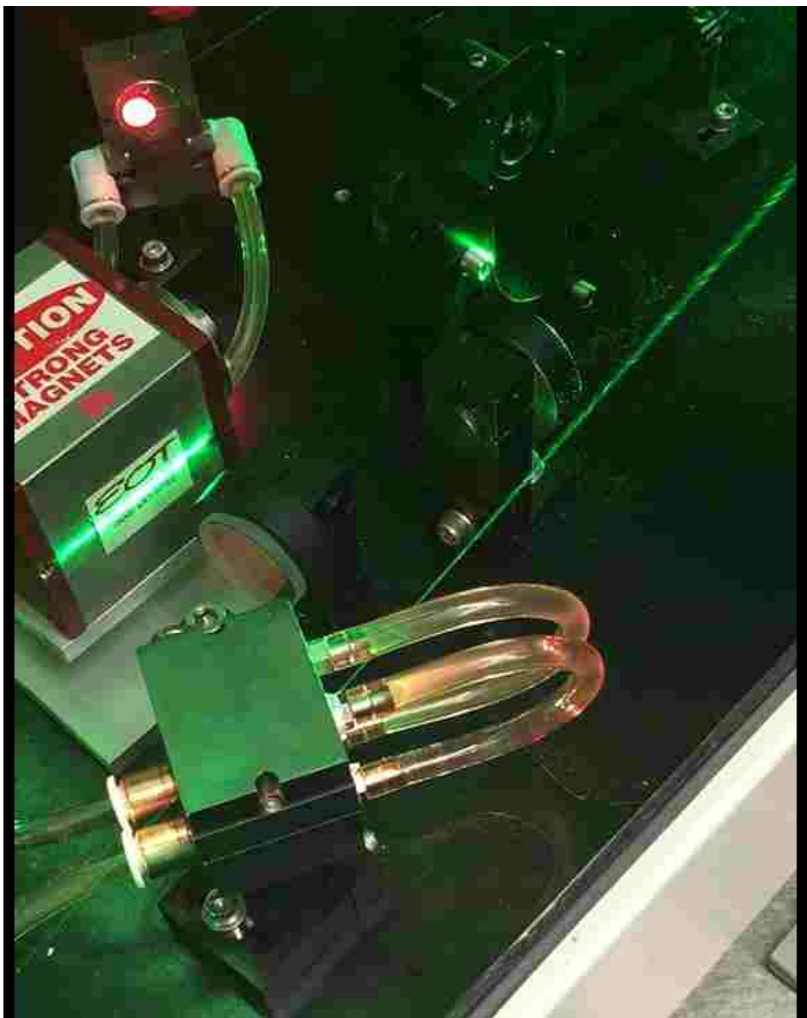
Fig. C. 14 The pump laser going through the Ti:sapphire crystal.
