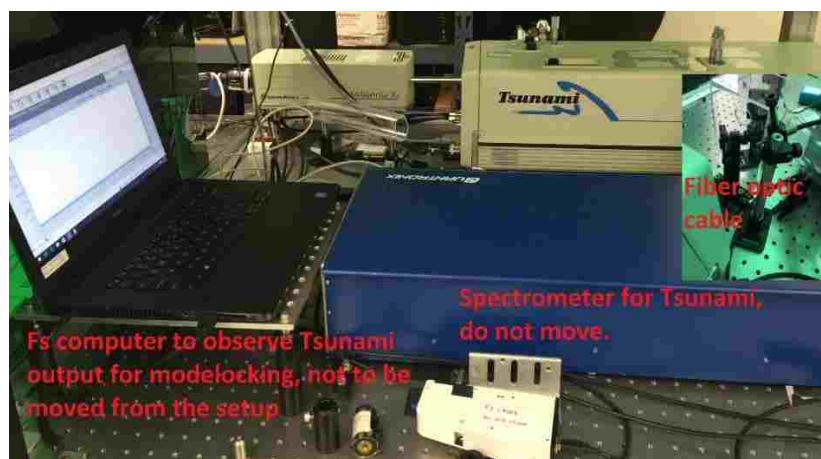
Fig. C. 3 Computer and the spectrometer to observe Tsunami laser output. There is no password on this computer. Spectrometer is dedicated to observe the mode-locking of Tsunami laser and should not be moved or used elsewhere.
