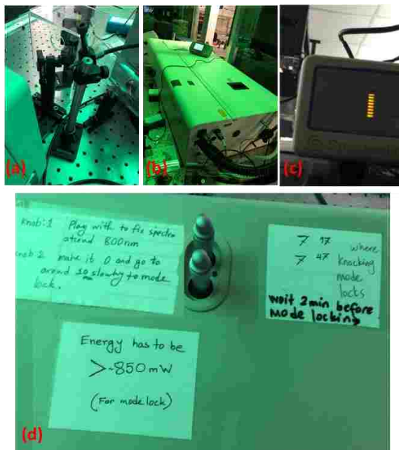
Fig. C. 18 (a) Fiber optic cable to detect output signal. (b) Regen body. (c) Photodiode signal from Tsunami output is critical for Terra laser start-up. Minimum 3 bars need to be ON to initiate the timing synchronization between the Terra laser and the Tsunami so that the Terra laser can turn on and Regen section can start. (d) Tsunami control reference parameters if fine adjustment is needed.
