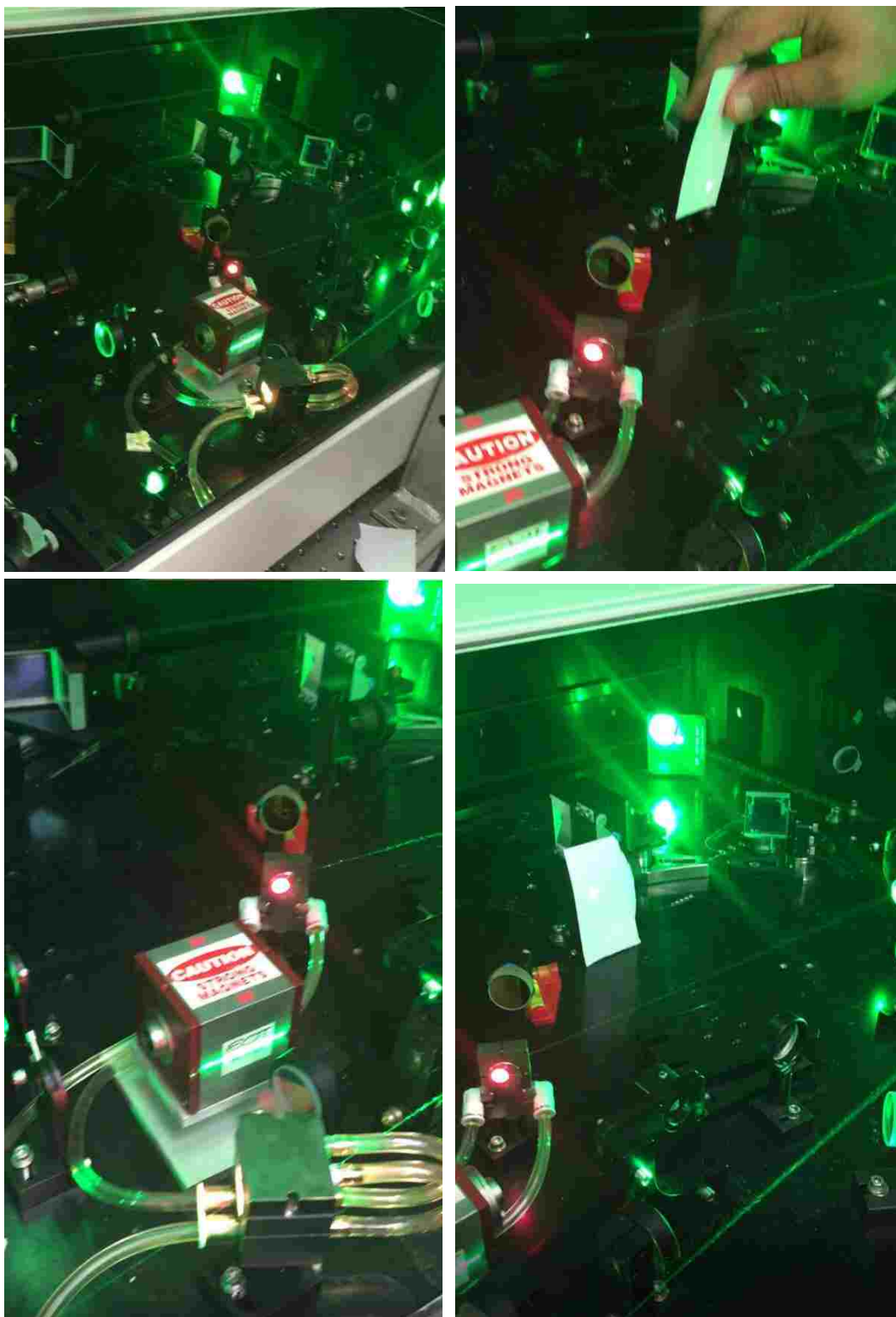
Fig. C. 13 Beam path inside Regen, seen through IR viewer. Refer to Fig. C. 6 for step-by-step guidance of beam alignment.
