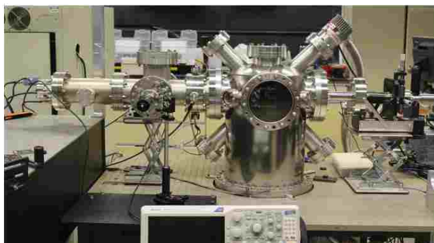
Fig. B.14 Schematic and image of the MCI system with ion deflection plates to avoid neutral deposition.
