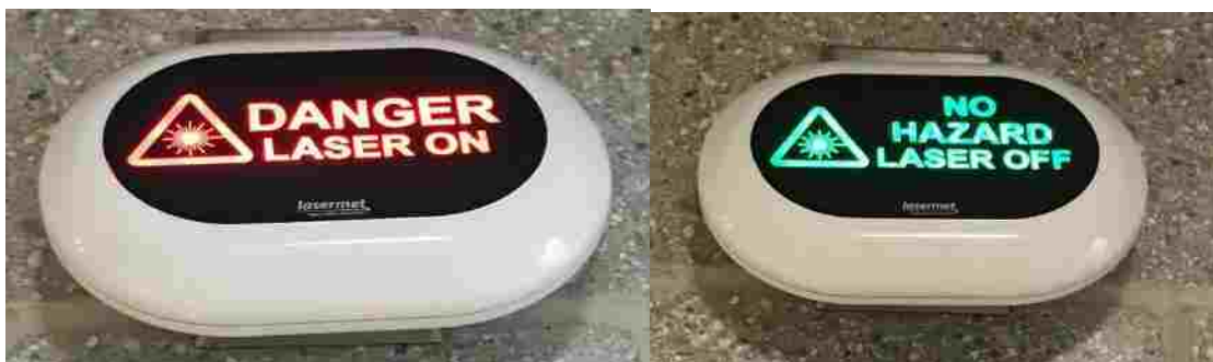
Fig. G.6 Illuminated indicator outside the room.
