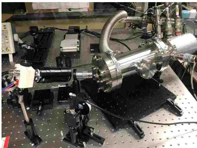
Fig. D.1 Cryogenic chamber for temperature dependence thermal conductivity measurement.
