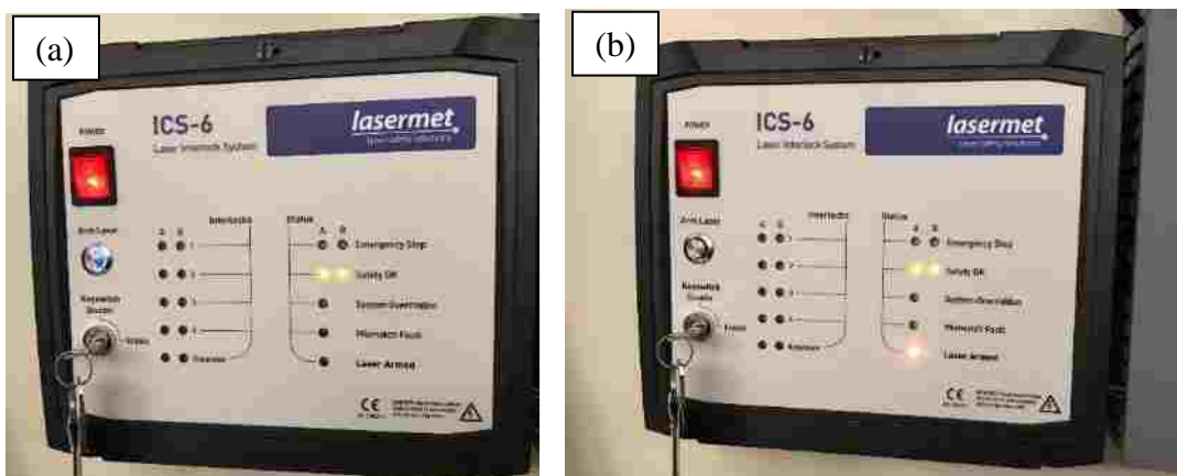
Fig. G.3 (a) The system is ready to arm. The blue LED is on. (b) The laser is armed by pressing the arm button. The laser arm LED is on.
