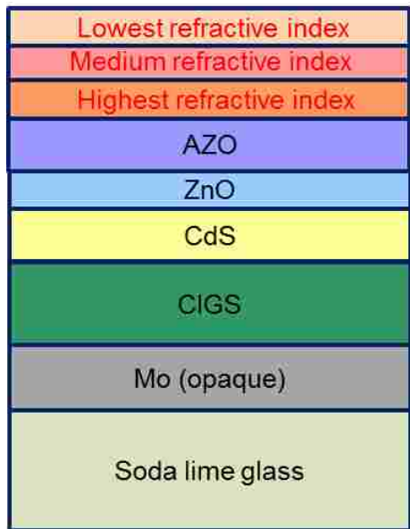
Figure 4. 8: Schematic diagram of ultra-thin CIGS solar cell with 3-layer graded ARC.
