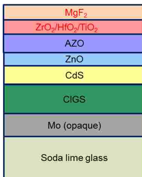
Figure 5. 1: Schematic diagram of ultra-thin CIGS solar cell with 2-layer ARC.
