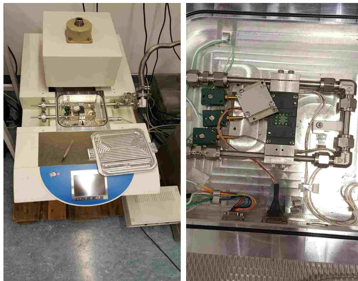
Figure 44. (a) View of the Linseis thermoelectric measurement System and b) close-up of the sample stage in the measurement chamber.
