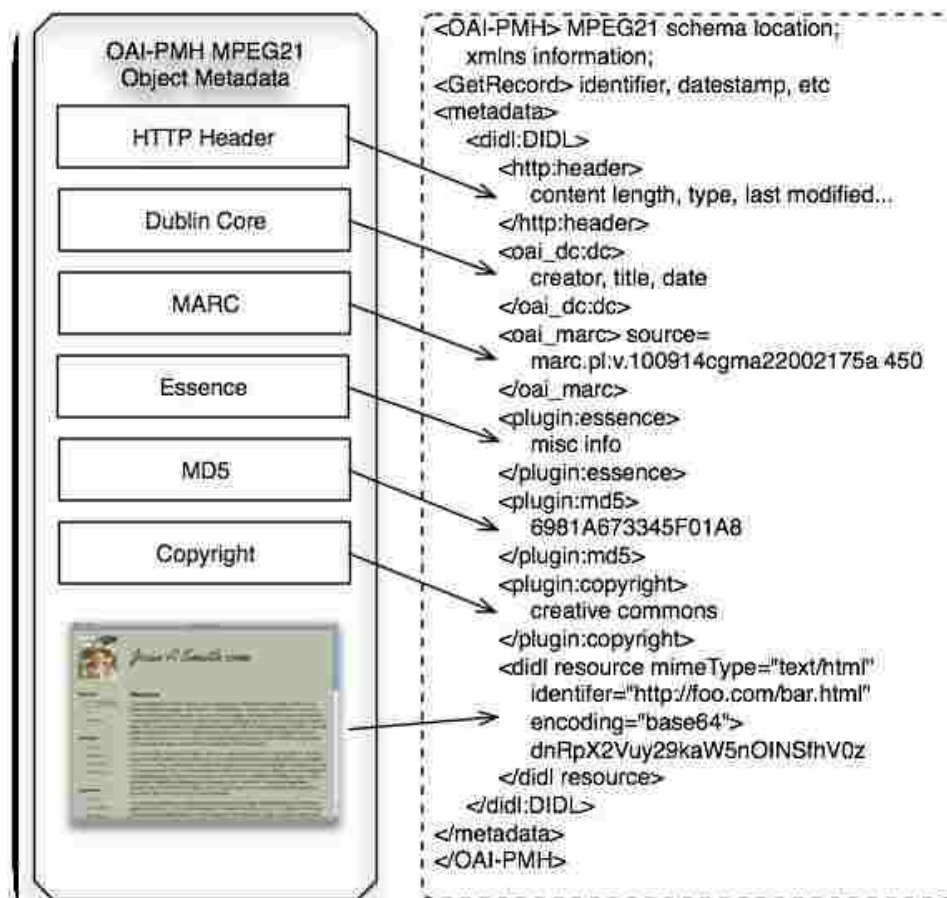
FIG. 57: Conceptual View of CRATE Object and XML Output in the MPEG-21 DID format.
