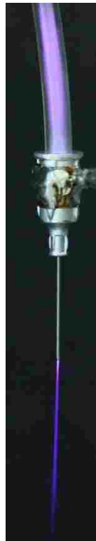
Fig. 1-1. A plasma jet by a single-needle electrode powered by 8 kV, 200 ns pulses at 500 Hz with helium flow of 200 SCCM, diameter of the needle tip is 0.508 mm.
