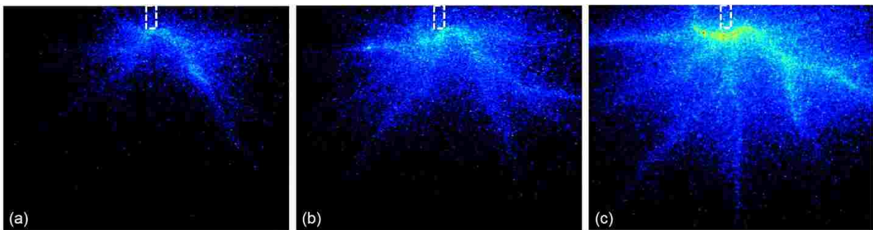
Fig. 4-8. Breakdown probability of air corona with varying amplitude (6 – 10 kV) for 200 ns pulses at 1 Hz, two repeated normal operations and one under excessive operation condition.
