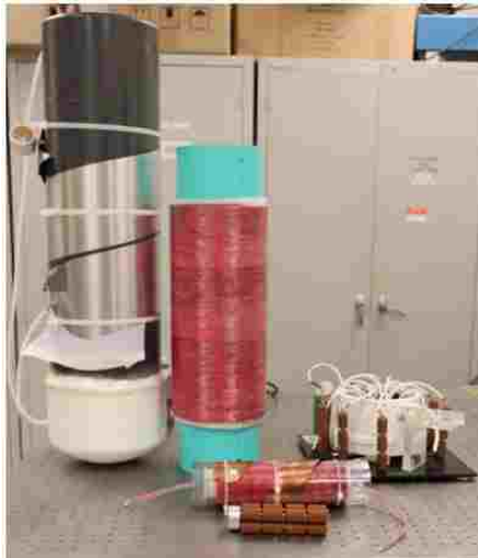
Fig. 41 Dual resonance pulse transformer designs
