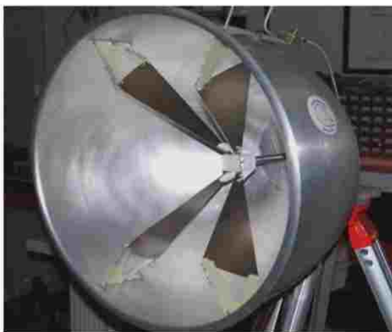
Fig. 2 Prolate spheroid antenna for the stimulation of neural tissue. The antenna is fed by a coaxial cable which is split to feed four arms [11].
