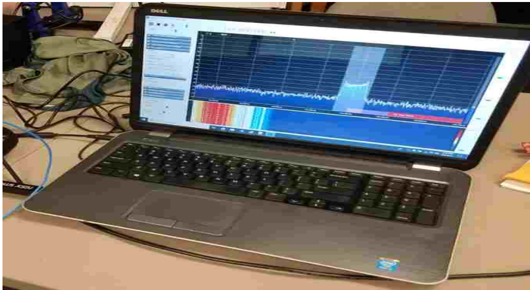
Fig. 37: RTL-SDR receiving "Hello World!" on 1200 AFSK
