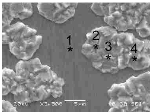
Fig. 4.5. Corresponding SEM Image for EDS P&S of Sample A-1 showing the location of the points used for further elemental analysis.
