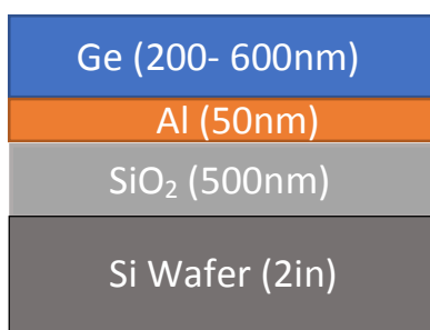
Fig. 5.1 Sample structure of aluminum-induced crystallization of germanium on silicon wafer with corresponding layer thicknesses.
