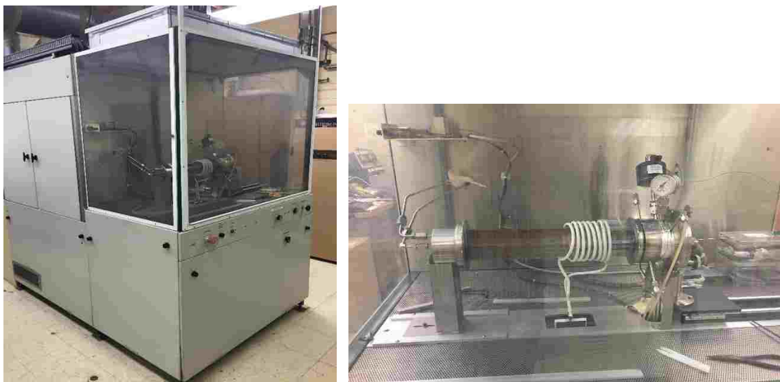
Fig. 2.1: Left: MOCVD Machine, Right: Horizontal reaction chamber located within the MOCVD machine
