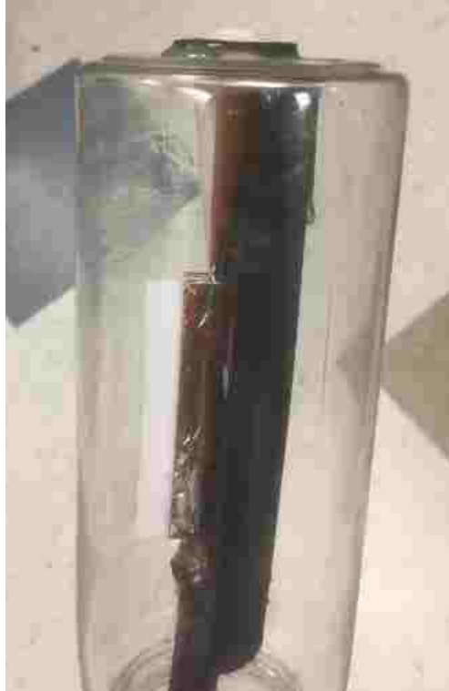
Figure 30: Antenna structure with a bottle housing
