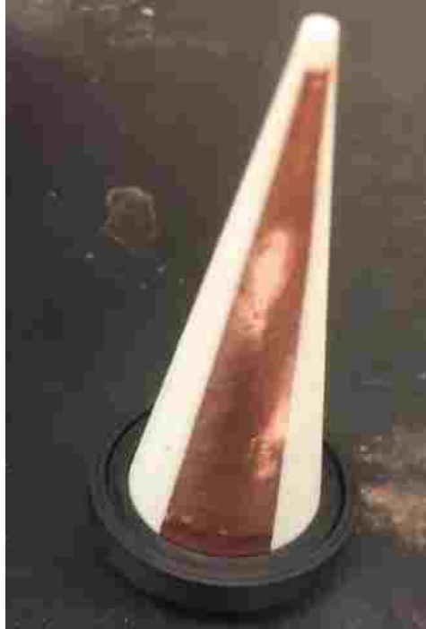
Figure 15: Constructed antenna model with resistor ring
