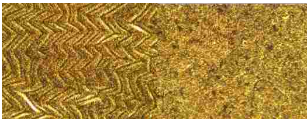
Fig 4.2 (a) Optical image of Indium layer with SiO 2 capping layer on Native Si/Mo-EB
