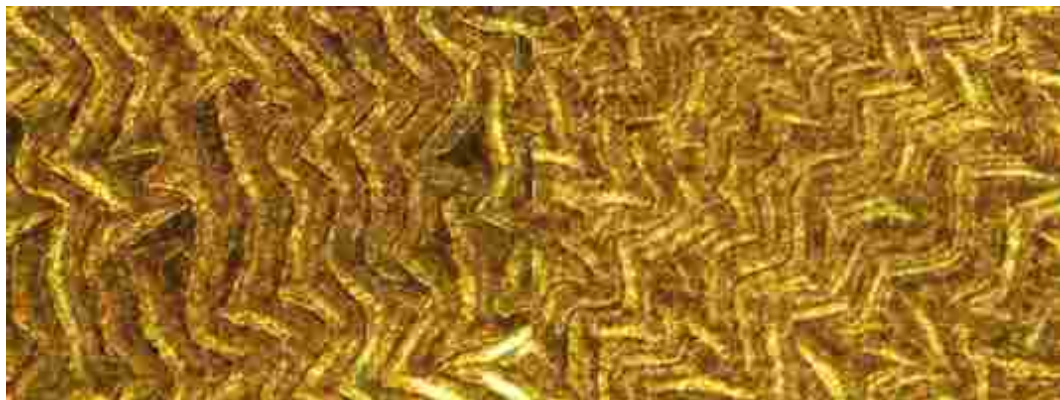
Fig 4.6(a) Optical image of Indium layer with SiO 2 capping layer on SLG/Mo-EB
