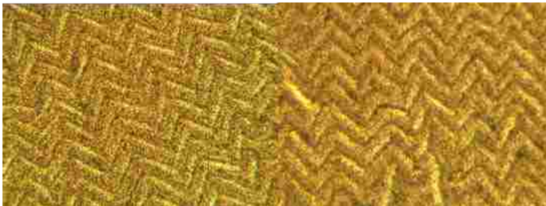
Fig 4.3(a) Optical image of Indium layer with SiO 2 capping layer on SLG/Mo-EB
