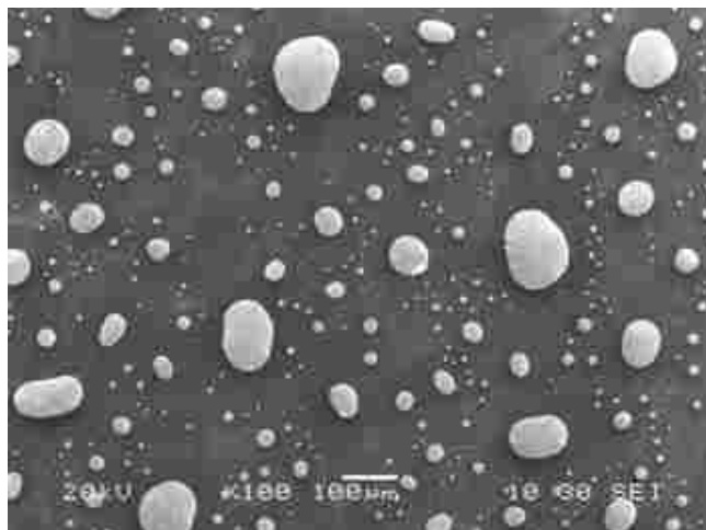
Fig 3.13. SEM image of Indium layer on SLG substrate with SiO 2 capping layer
