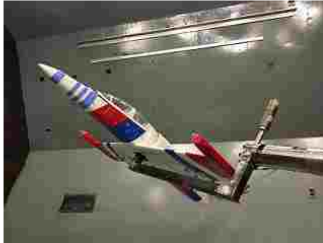
FIG. 1: Model Plane on Free-to-Pitch Rig
