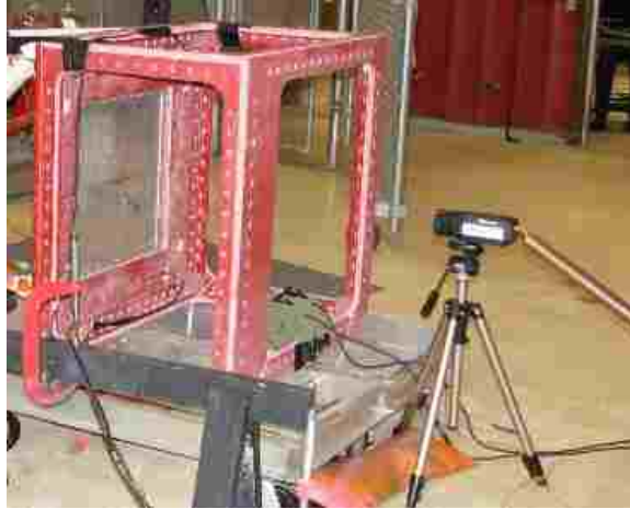
Fig. 11. Photograph of IR camera used at the testbed to capture backside temperatures [3], [14]
