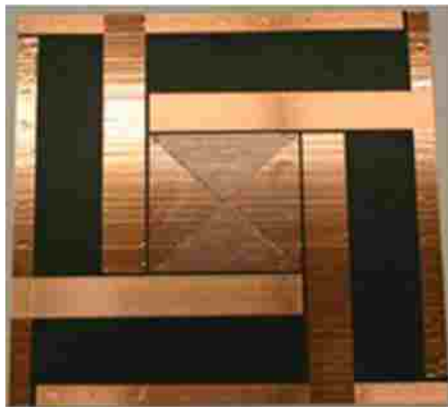
Fig. 9. Actual Test Panel with 7-inch SansEC (shown unpainted) [3], [14]
