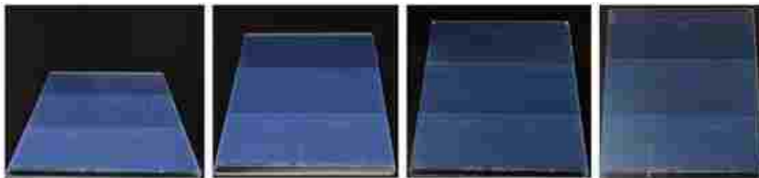
Fig. 5.3. Photographs of 200 nm nanoparticles coated glass slide taken with camera lens axis positioned at 30^\circ , 45^\circ , 60^\circ , and 90^\circ (left to right). The glass slide was coated by one, two, and three coats (top to bottom each covering one third of the slide).
