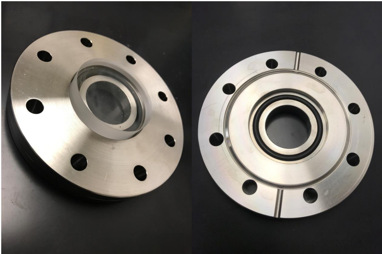
Figure 4 fused quartz window O-ring sealed when bolted to the chamber
